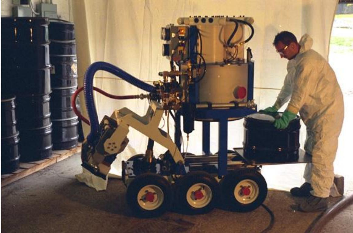
Figure 15. PENTEK Moose® Remotely Operated Floor Scabblers.
