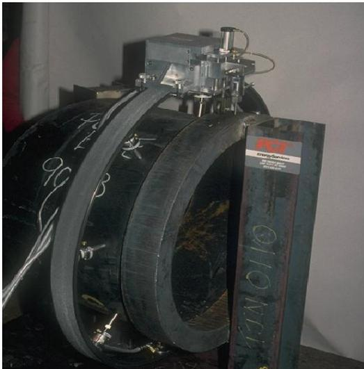
Figure 12. Track Cutting System for Plasma or Oxy-Fuels.
