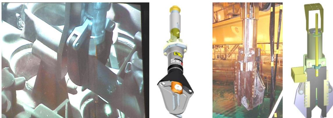
*Figure 3. Shearing tools used to cut the core spray system and flat bars on the core grid.*
