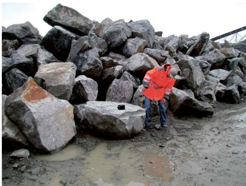
Figure 8-5 If there is no equipment for weighing the blocks, the blocks can be measured and the weight subsequently calculated. Shown here by blocks that are well-suited for interlocking surfaces. (Rock for Bykaia, Longyearbyen. Photo: Norconsult).
