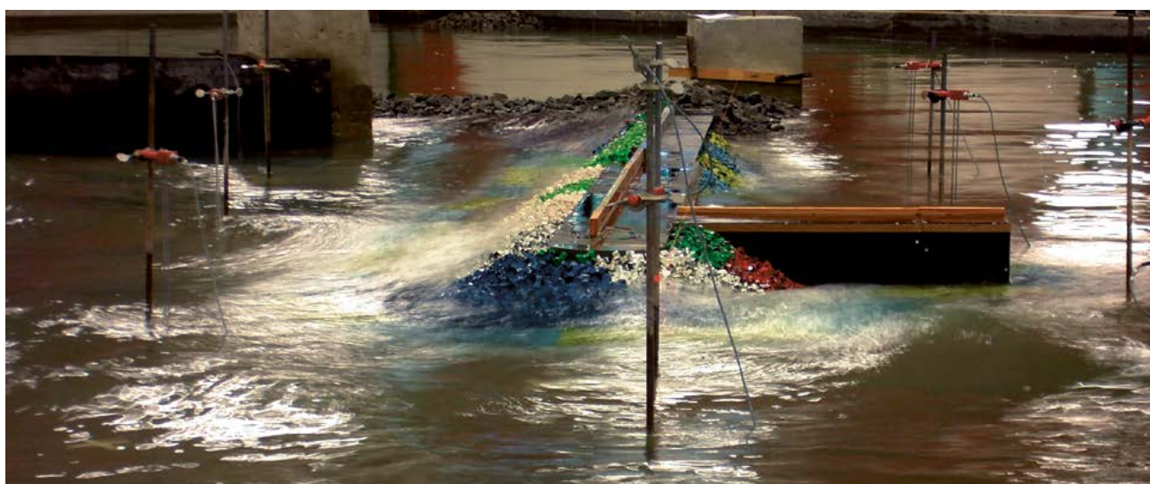
Figure 5-6 Example of 3D experiment in wave basin, scale: 1:58, crest elevation +7 m, sea bottom -9.5 m, water level +1.5 m, H_{s,100} = 5.1 m, T_p = 16 s, X_{bloc} = 10 t. (Photo: DHI).
