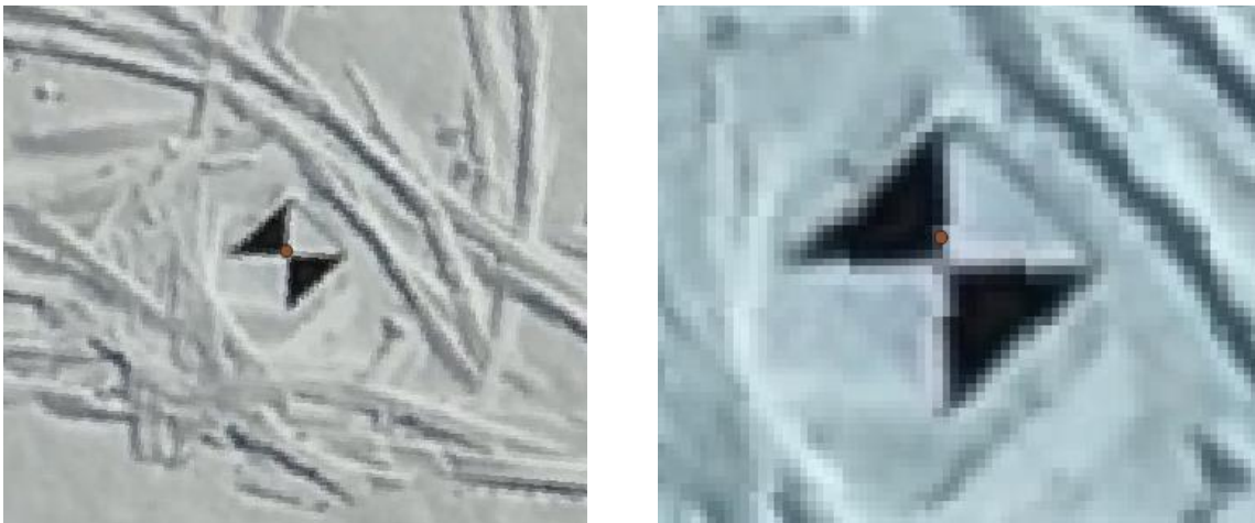
Figure 3.5.1-2: Orthophoto with control points, showing georeferenced differences for the two independent datasets, left side, reference dataset#1 M300, right side, dataset#2 Phantom 4
