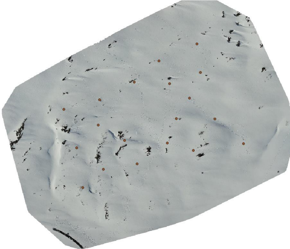
Figure 3.3.2-2: Orthophoto with visual GCP's Breiddalen#1 dataset (DJI M300 RTK), made with the MOD_ODM procedure
