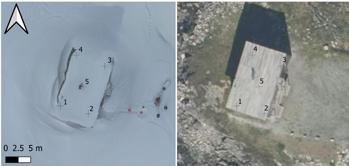
Figure 2.8-1: Location of reference points on the roof of Fonnbu research station where height values are extracted from each flight.
