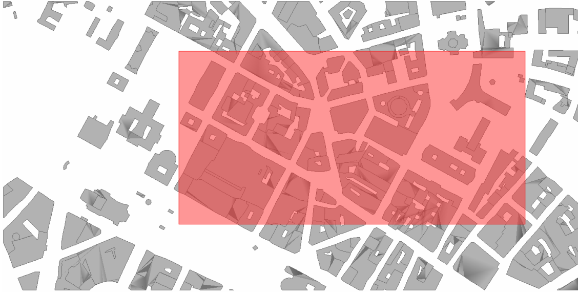
Figure 6.6 The area over which metrics are calculated based on a uniform distribution of interrogation points is shown in red. The full urban area of the simulations used for parameter investigations is shown in gray. The global wind direction is from left (west) to right.
