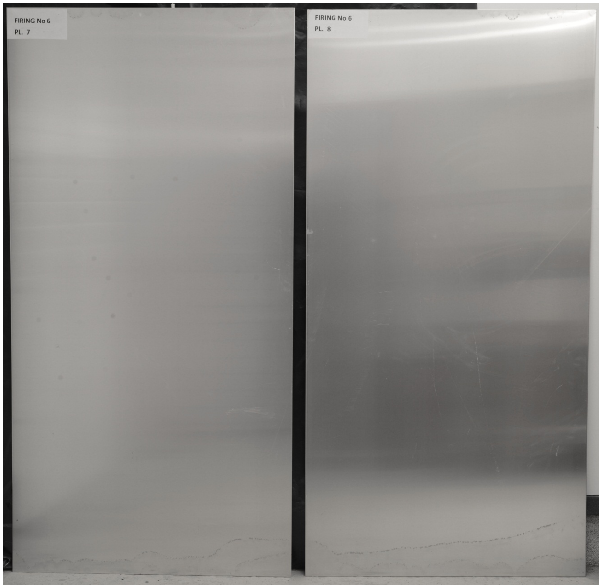
Figure App C. 29 Witness plates No 7 and No 8 from firing of shell No 7 filled with MCX-8001 composition.
