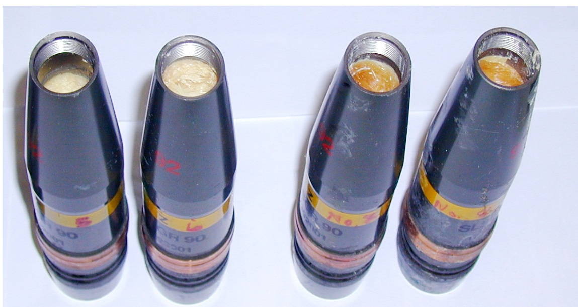
Figure 2.4 TNT filled shells, left with MCX-6002 and right with MCX-8001 composition.
