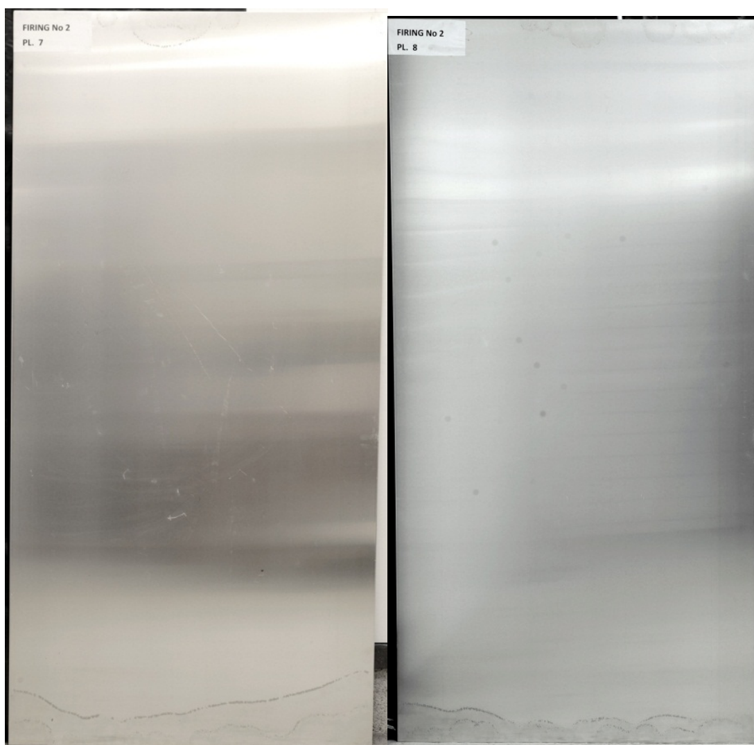
Figure App C. 12 Witness plates No 7 and No 8 from firing of shell No 6 filled with MCX-6002 composition.
