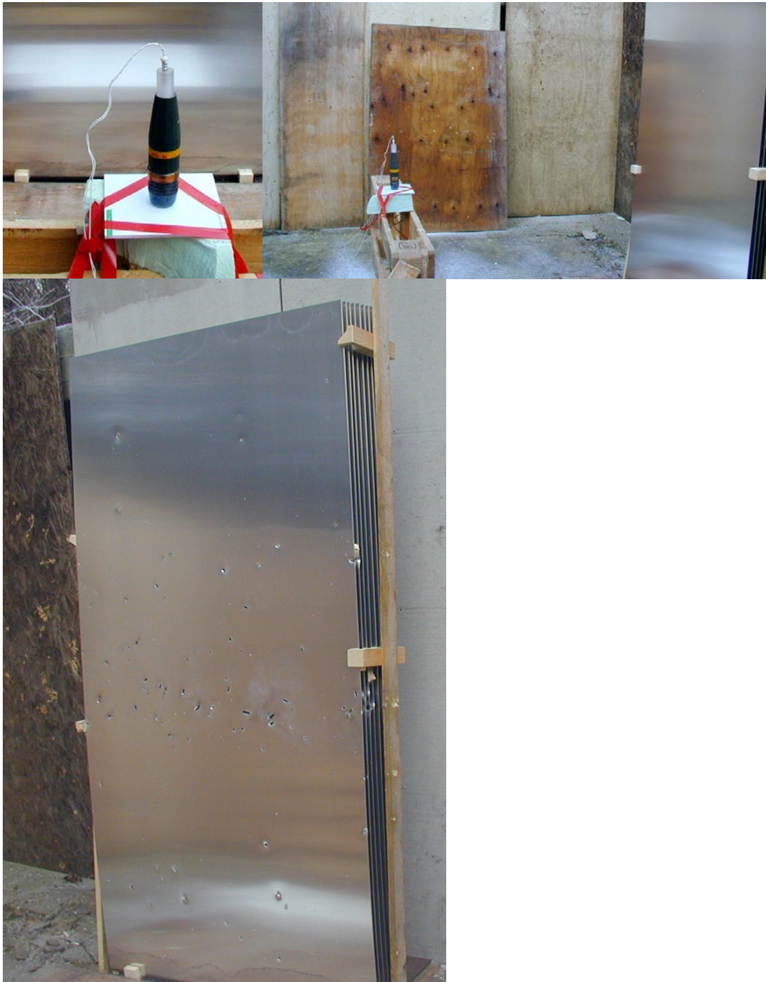
Figure 3.4 Pictures from different angles of shell No 6 before firing, and of the stack of witness plates after firing.
