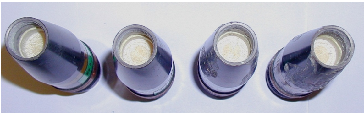
Figure 2.9 The DNAN filled shells after modification: from left No 1 and No 2 containing MCX-6100 composition, No 3 and No 4 containing MCX-8100 composition.
