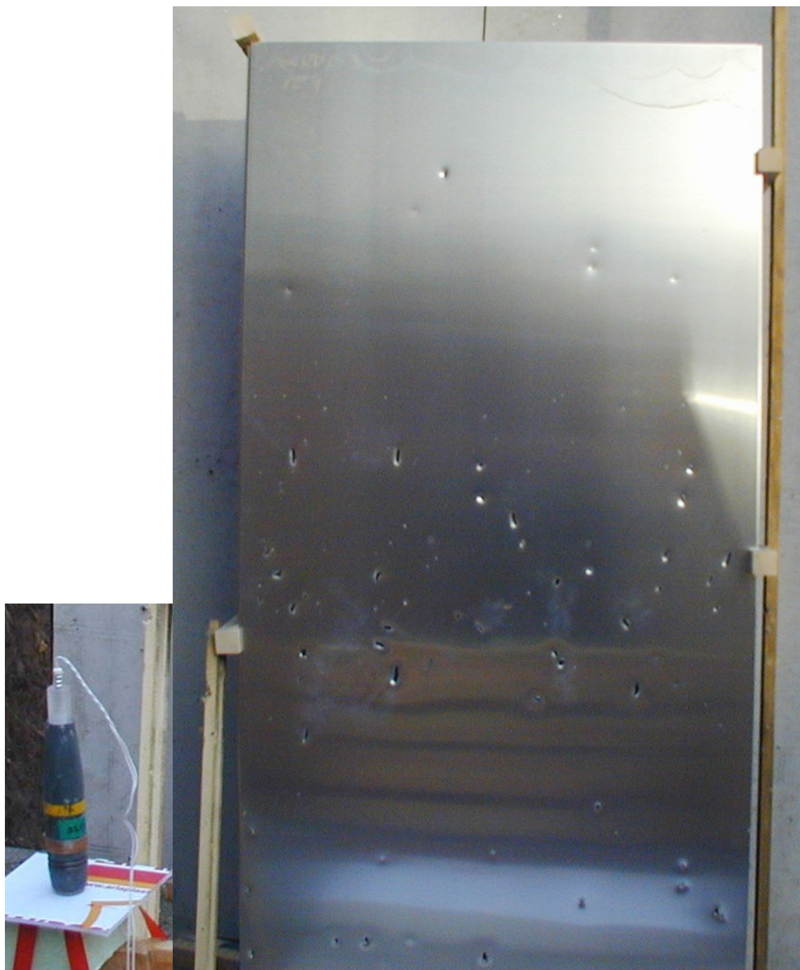
Figure 3.7 The figure shows a picture of shell No 4 before firing and a picture of the stack of witness plates after the firing.
