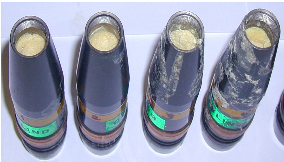
Figure 2.3 DNAN filled shells, with MCX-6100 number 1 and 2 from left and with MCX-8100 composition number 3 and 4 from left.
