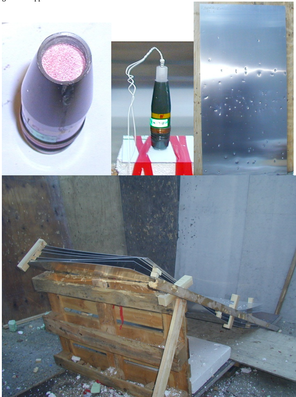
Figure 3.17 Pictures from firing No 7 of shell No 5 filled with MCX-6002 composition.
