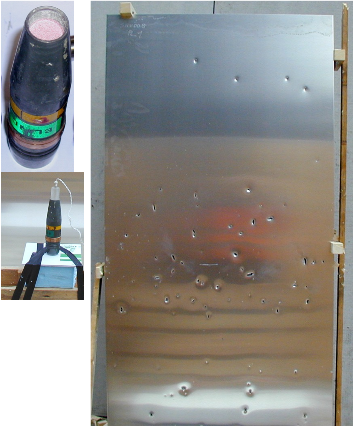
Figure 3.20 Pictures from firing No 8 with shell No 3 filled with MCX-8100 composition.
