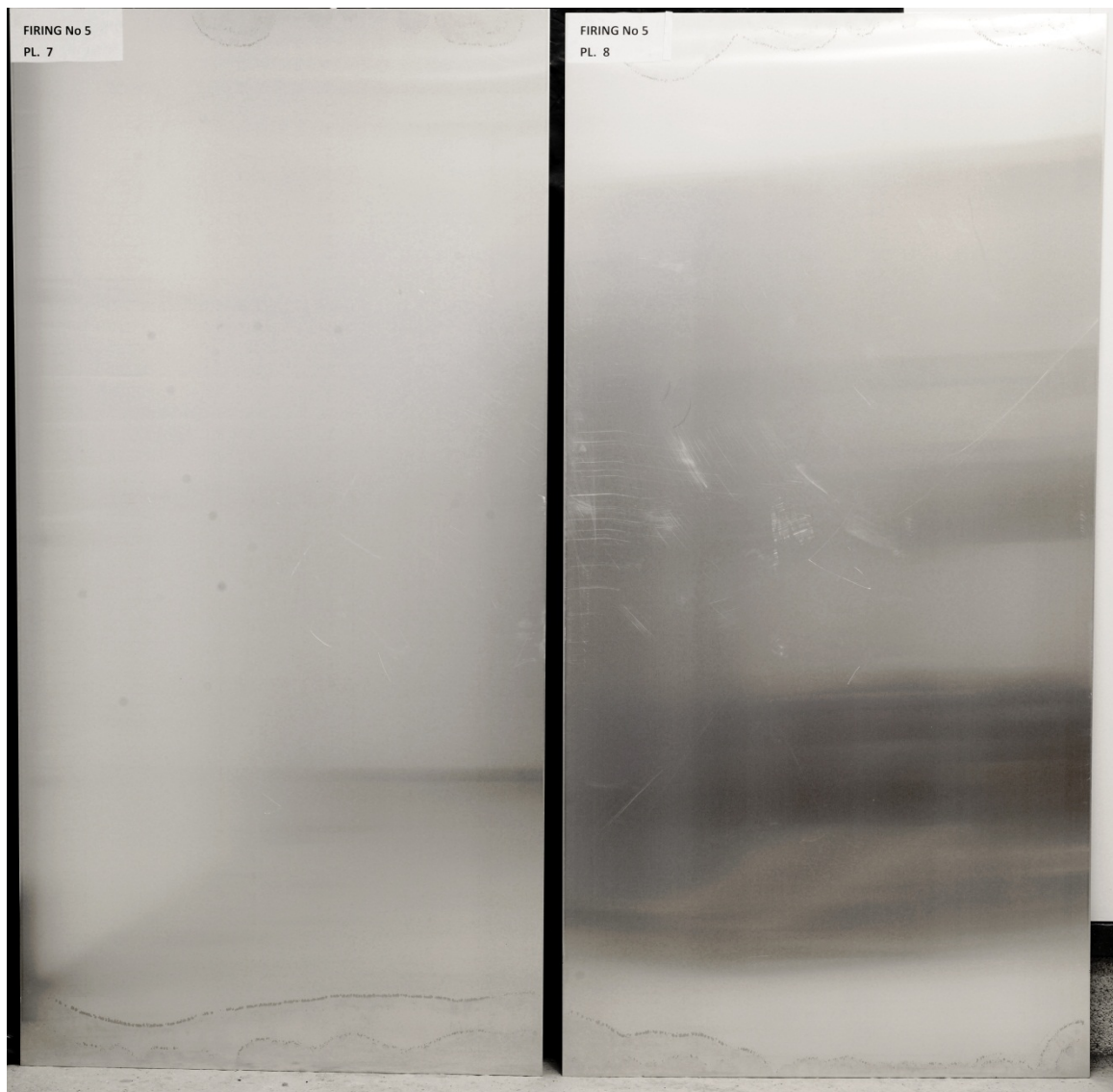
Figure App C. 25 Witness plates No 7 and No 8 from firing of shell No 10 press filled with GA/BAMO/IPDI/HMX Sats 432/13 composition.
