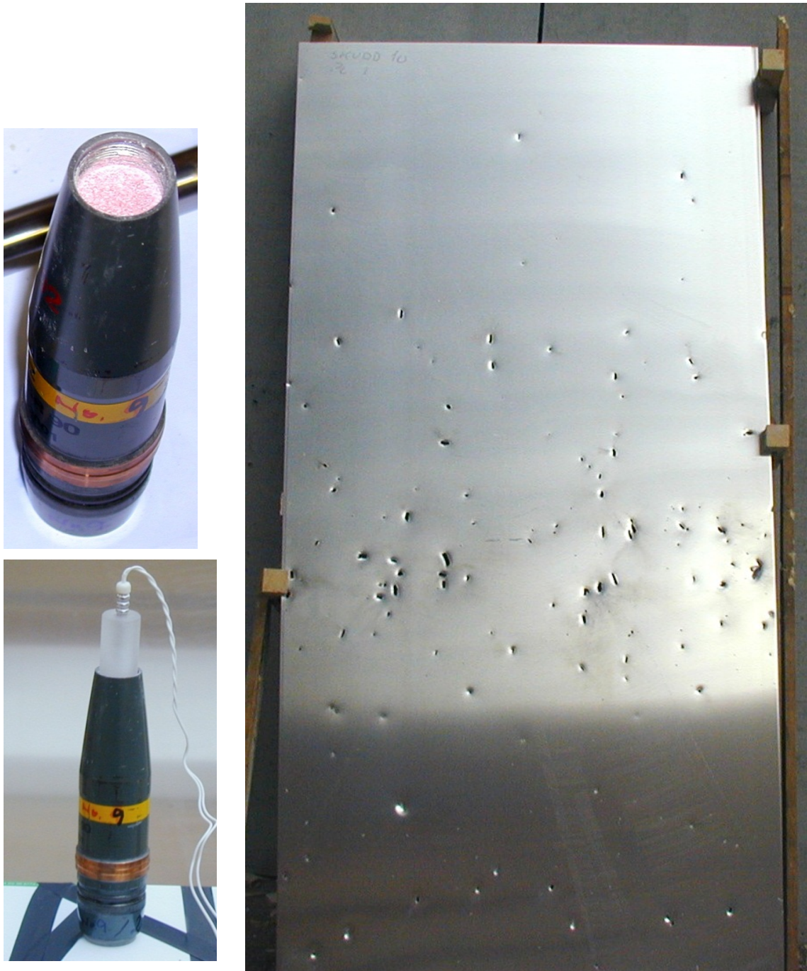
Figure 3.26 Pictures of the shell before firing and of the stack of witness plates after firing for shell No 9
