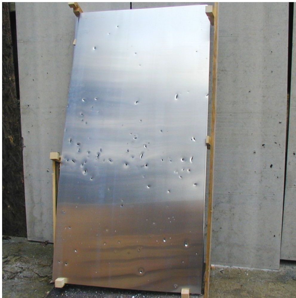
Figure 3.1 The witness plate stack after detonation of shell No 8 filled with MCX-8001 composition.
