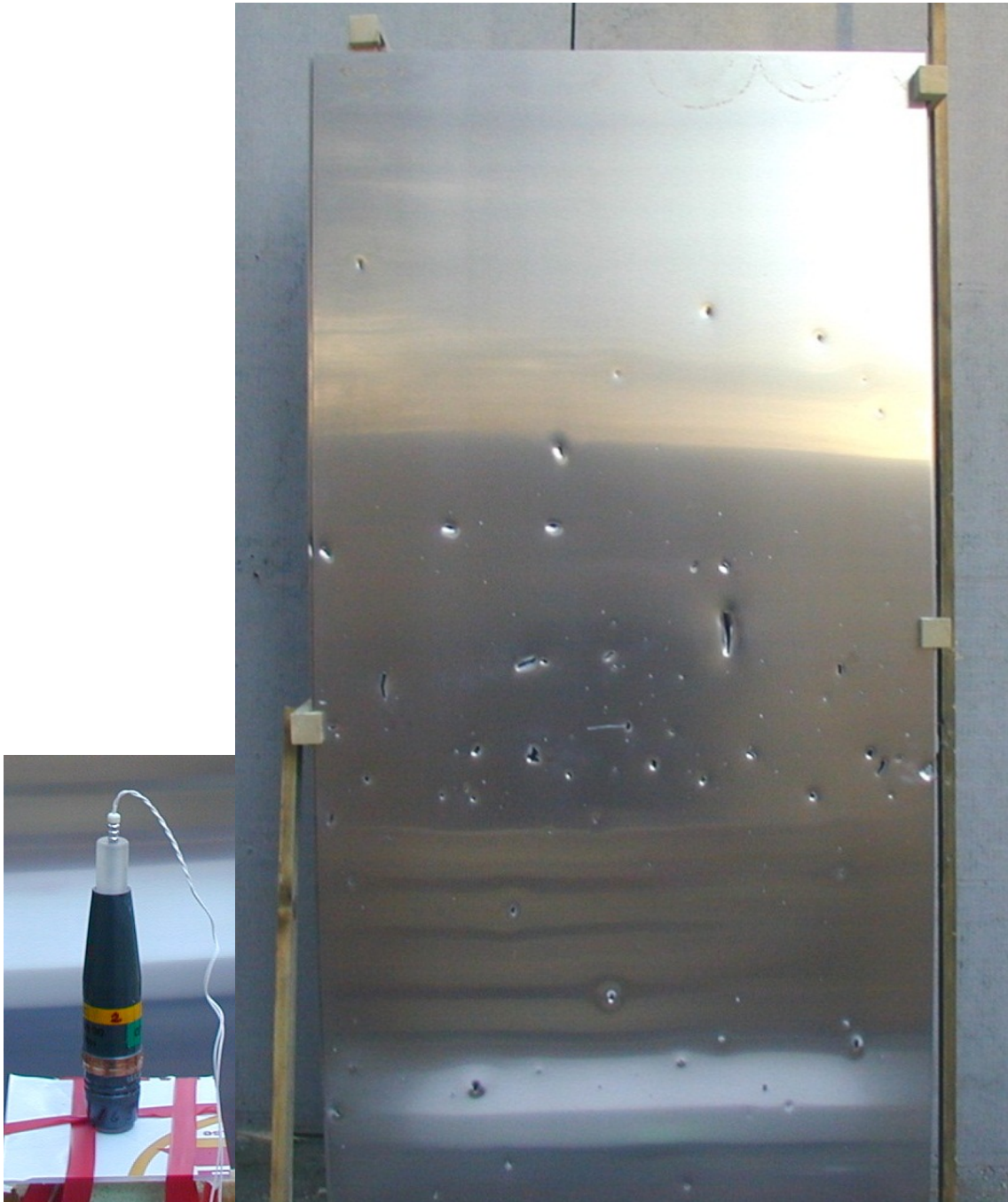
Figure 3.10 The Figure shows pictures of shell No 2 before firing and the stack of witness plates after firing.
