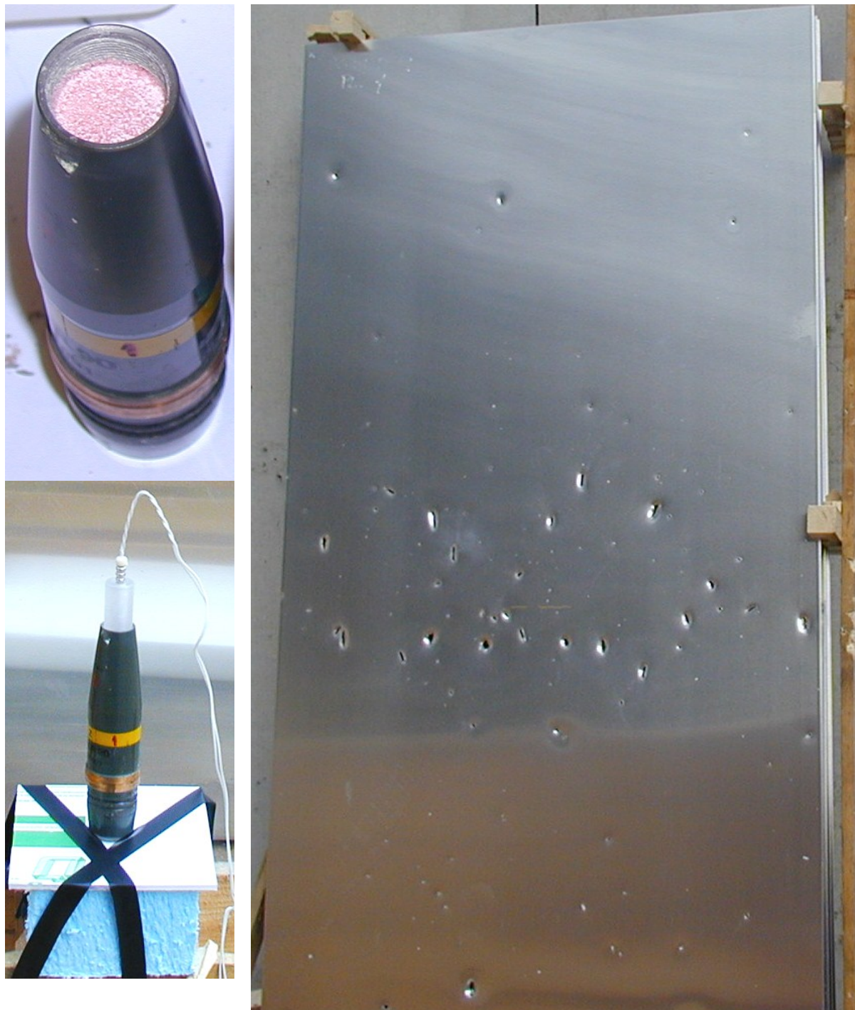
Figure 3.23 Pictures from firing No 9 with 40 mm shell No 1 containing MCX-6100 composition.
