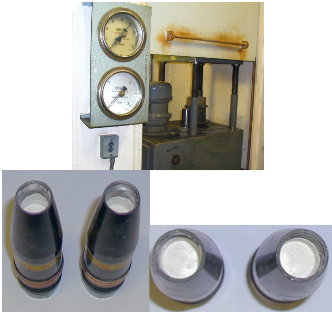
Figure 2.11 The pictures show the press used for filling, and the shells after being filled with Sats 400/13 and Sats 432/13 compositions.
