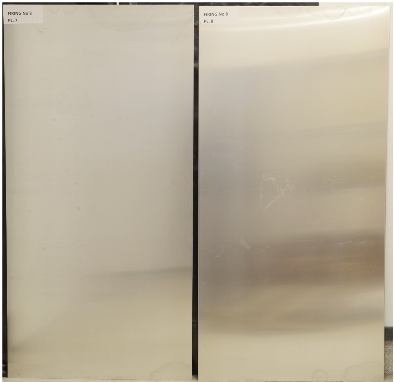
Figure App C. 37 Witness plates No 7 and No 8 from firing of shell No 3 filled with MCX-8100 composition showing no fragment hits.
