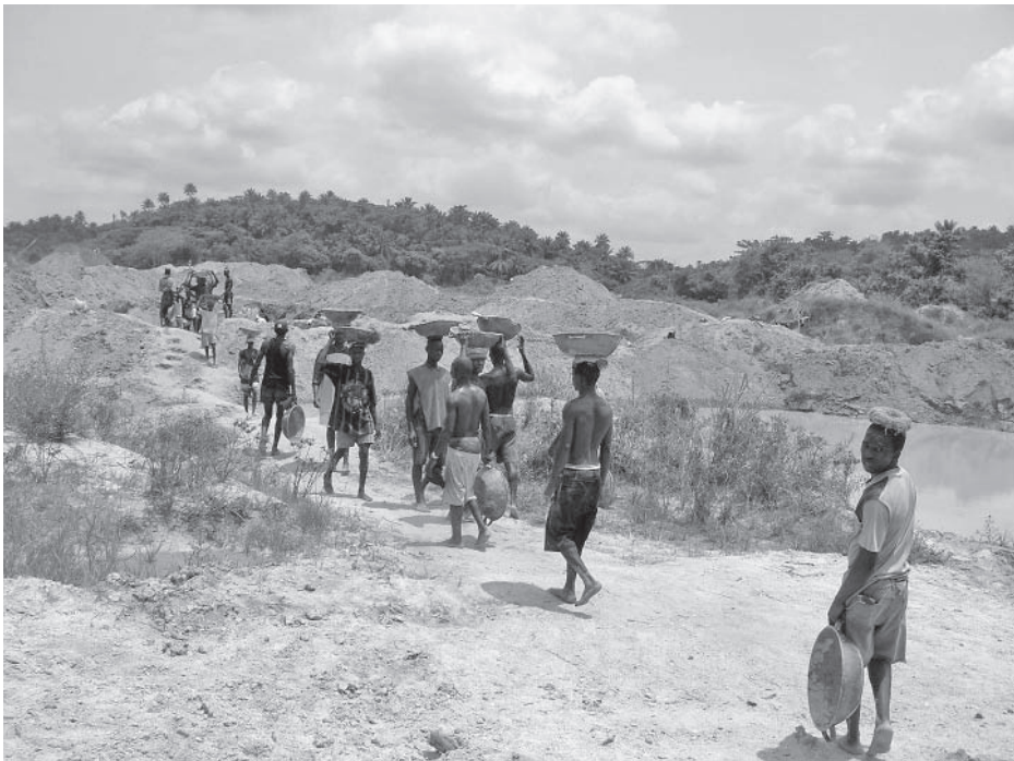
Figure 2.1 Direct workers carrying gravel to the site for washing
