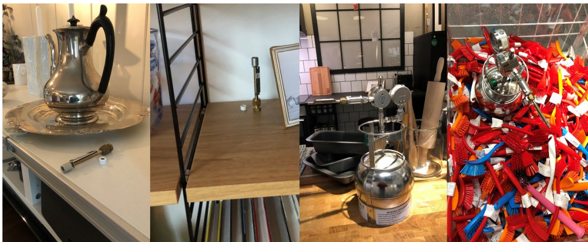
Figure 5: Air sampling in indoor residential and public environments. Tenax TA tubes as passive air samplers (2 images left) and active air samplers (2 images right). (Photo: Heidi Eikenes, Helene Lunder Halvorsen, Pernilla Bohlin-Nizzetto, NILU.)
