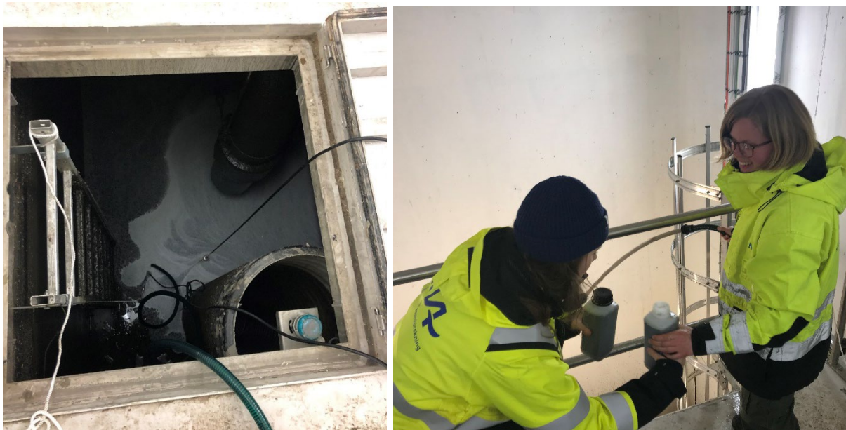
Figure 10: Sampling of tunnel wash water during a tunnel wash in the Smestad tunnel pump station. (Photo: Elisabeth Rødland/Sondre Meland, NIVA)
