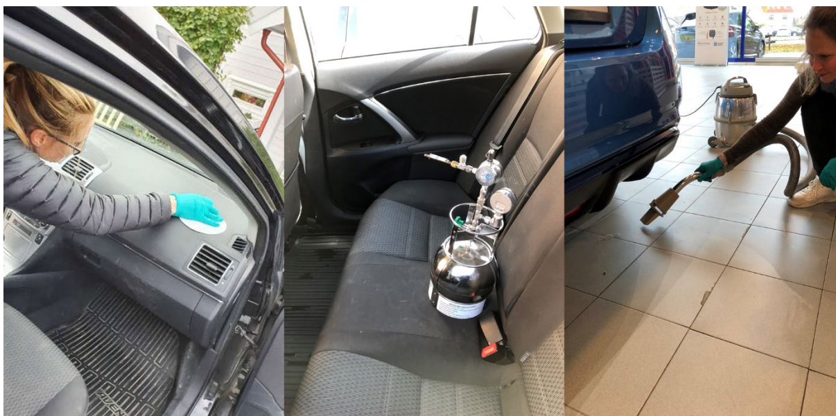
Figure 1: Sampling of settled dust and air in cars and car retailers. (Photo: Heidi Eikenes, Helene Lunder Halvorsen, Pernilla Bohlin-Nizzetto, NILU.)
