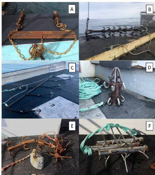
Figur 26 Eksempel på sokneredskaper brukt for å fiske opp mistet redskap på hardbunn. A. Double pircupine grapple, B. Hook grapple, C. Span drag, D. Cylinder block grapple with additional chain for weight, E. Cylinder block grapple with additional chain for weight, E. Cylinder-type grapples with a boulder for weight, and F. Porcupine-type grapple. Adapted from Goodman et al., 2021 and McIntyre et al., 2023.
