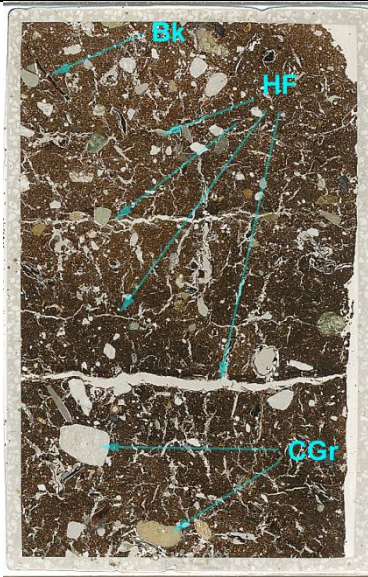
Fig. 33: Scan of M18413 (18161; 10220); horizontally fissured (HF) probably diffusely layered minerogenic peaty deposits with coarse gravels at the base (CGr), much rooting and many fine charcoal (Figs 34-37), as well as woody materials including bark (Bk; Figs 38-39). Frame height is ~75mm.
