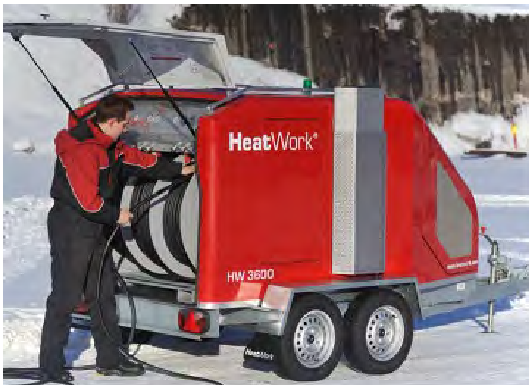
Figur 9-18 HeatWork Ice Guard System (Foto: HeatWork)
