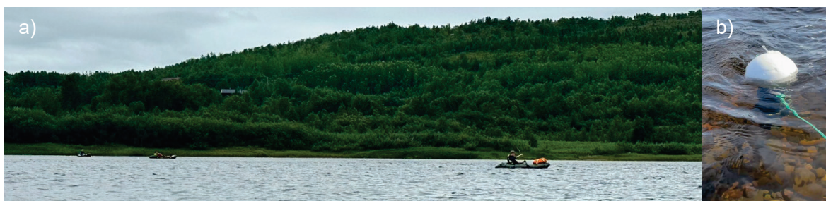
Figure 5. Manual tracking survey with three out of 4 packrafts in parallel (a), each with a receiver suspended from a buoy towed behind the packraft (b). Photos: K. Ø. Gjelland
