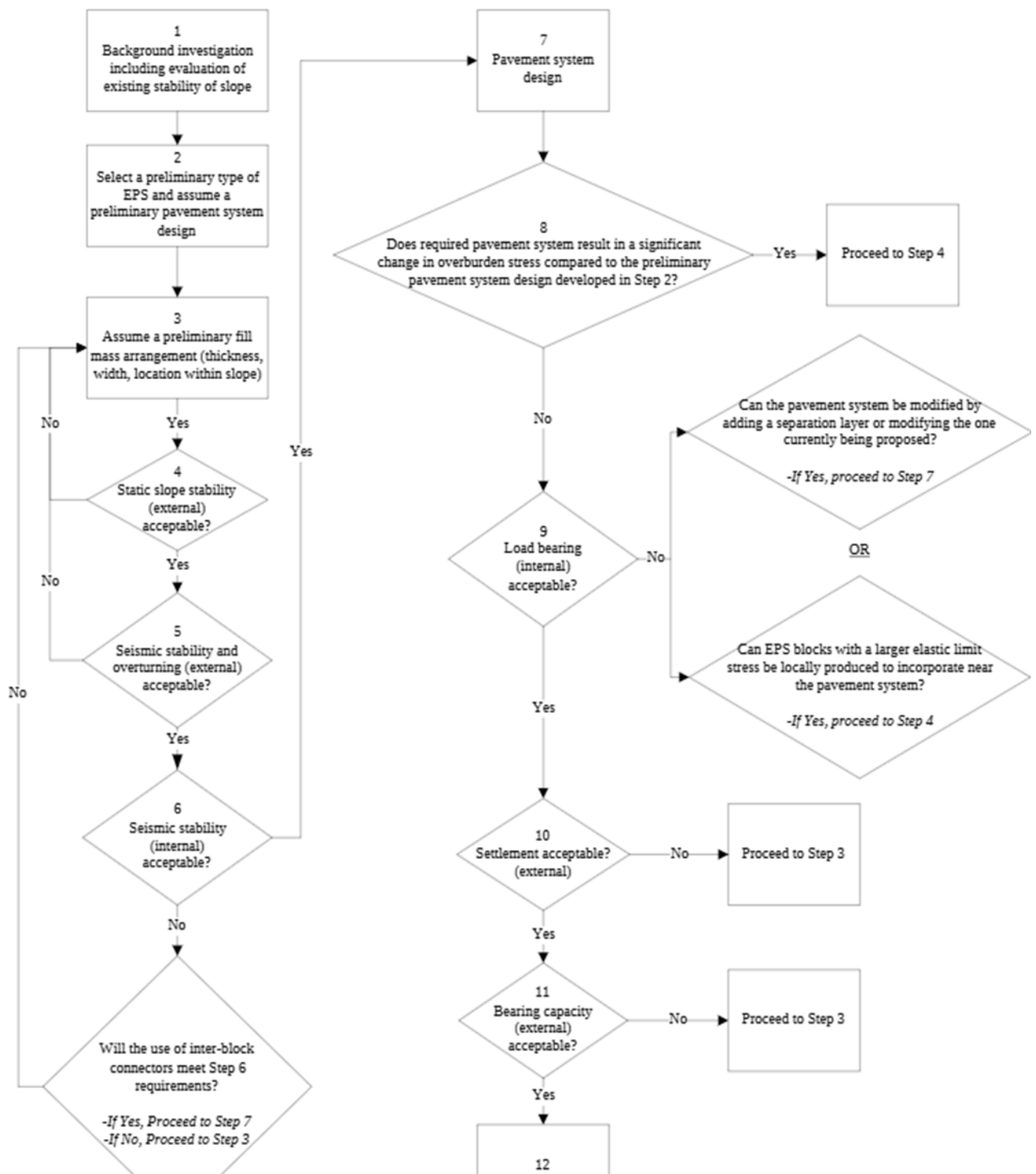
Figur 3. Guidelines for Geofoam Applications in Slope Stability Projects (2013). The National Academies Press
