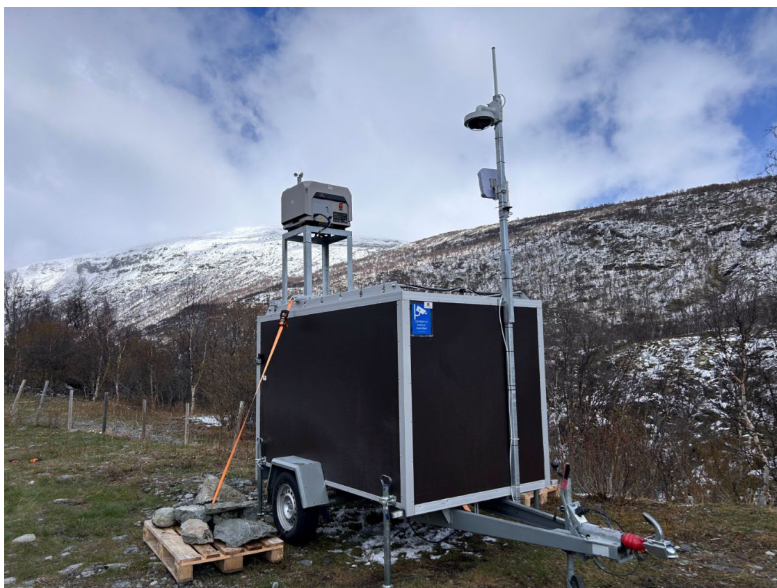
Figure 6: NPRA's first operational drone docking station in Drivdalen is a modification of the set-up used at Ørskogfjellet (photo: Halgeir Dahle, NPRA).
