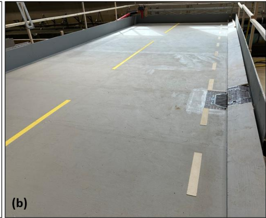
Figure 9 - a) The road markings used for the test are highlighted, and b) the setup after the addition of road markings
