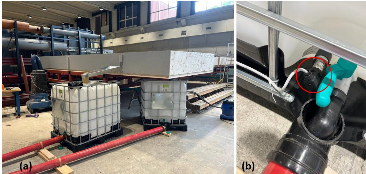
Figure 6 - a) Containers collecting water from the tests, and b) a pressure sensor installed on each container
