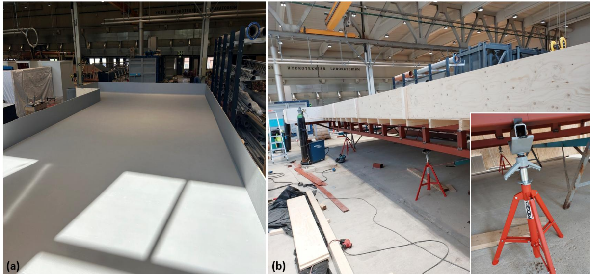
Figure 4 - a) The surface of the wooden frame which represents the road surface in the tunnel, and b) four adjustable jacks are used to hold the frame while having the option to change the slopes
