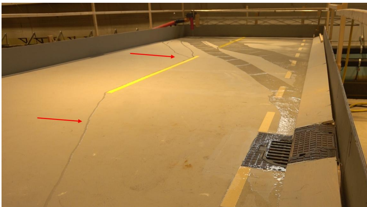
Figure 18 - A stream of water forming along the middle road markings, passing the drain. The test was performed on a 5 percent slope and a 0.3 L/sec discharge.
