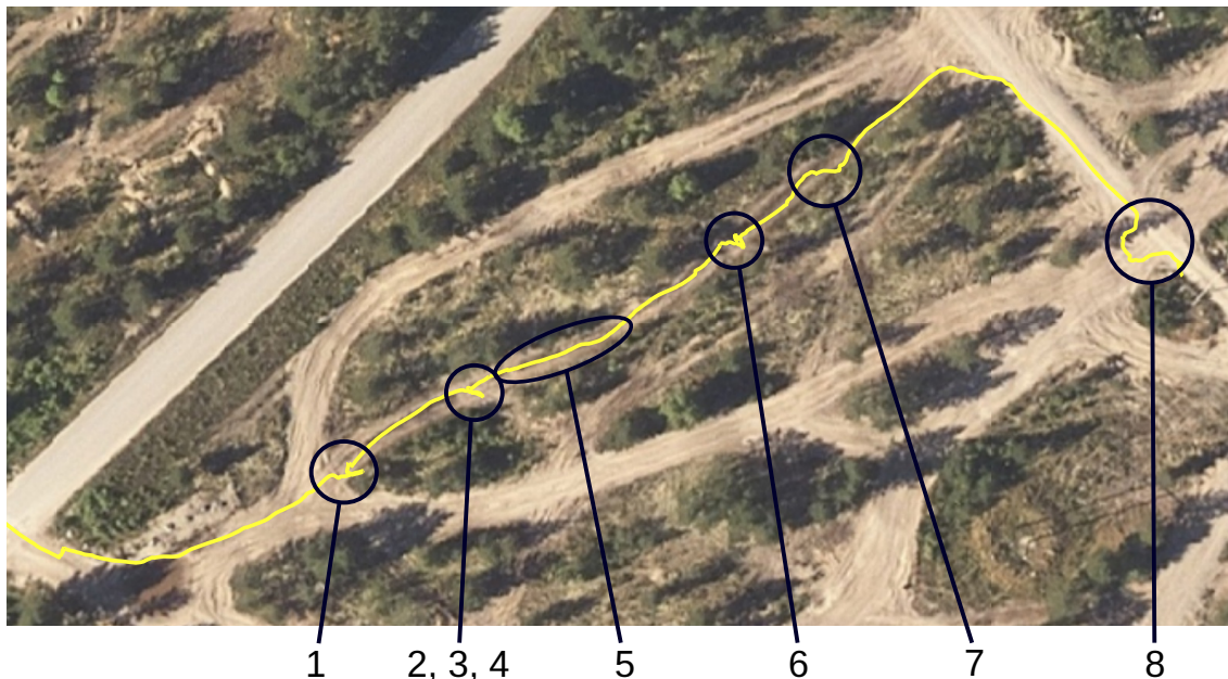
Figure 5.11 Experiment 4 – A closer look at the driven path through a narrow vehicle trail section. The numbers indicate issues or manual interventions.
