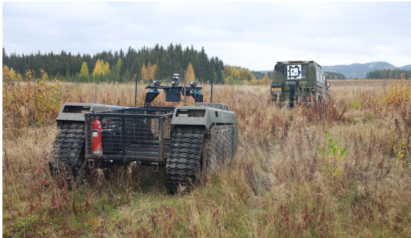
Figure 4.1 LandX21: Tor following a lead vehicle as it did during the logistics demonstration. The AprilTag on the back of the lead vehicle is what makes Tor able to track the vehicle using a camera.
