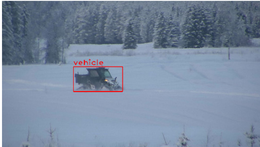
Figure 3.23 Example of image-based detection using Yolo from 2018. The detected vehicle is our old UGV Olav, a Polaris Ranger.
