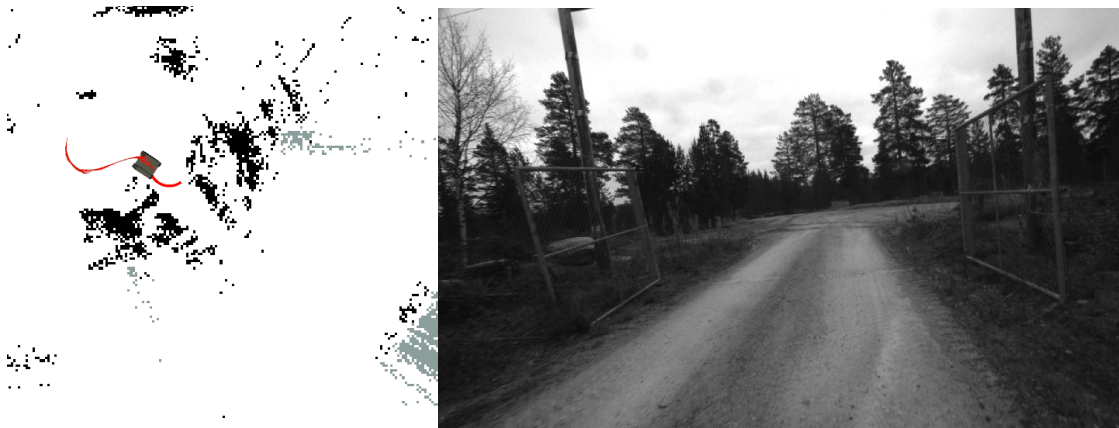
(a) Obstacle map with UGV in front of the gate. The gate is too narrow to pass in the obstacle map (b) Simultaneous view from Tor. The gate is clearly wide enough to pass.
