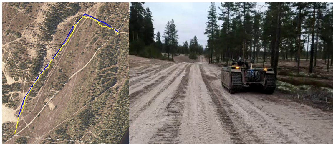
(a) Input route (blue) and driven path (yellow), starting from the south. (b) Tor during experiment 2 on the vehicle trail and hugging the tree line.
