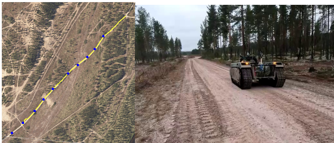
(a) Results from following a dirt road. Input waypoints in blue and driven path in yellow.
