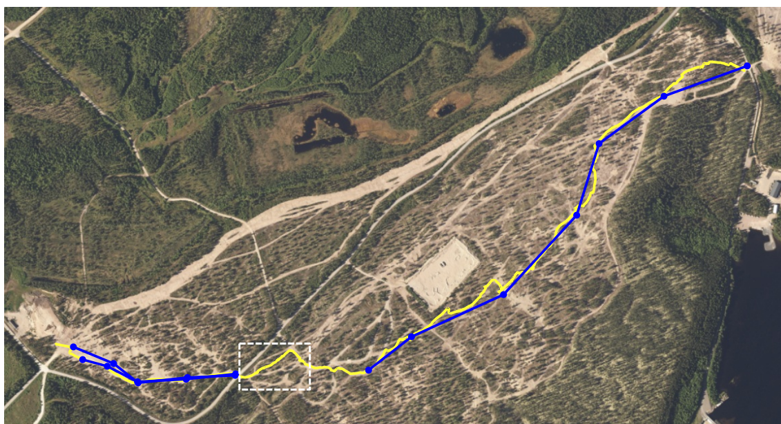
Figure 5.10 Experiment 4 – Input routes in blue and driven path in yellow. The start position was to the left. A closer look at the area within the rectangular marking can be seen in Figure 5.11.
