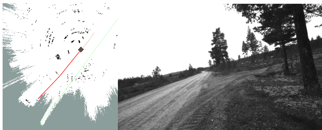
(a) Obstacle map with UGV position, planned trajectory and goal point in blue.
