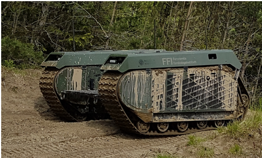
Figure 2.1 Our Milrem Themis, Tor, without sensors or payload.
