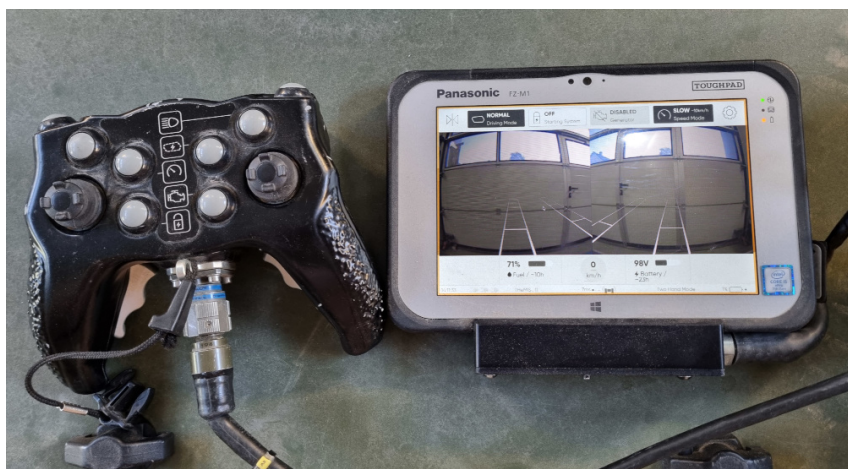
Figure 2.2 The hand controller and tablet for controlling the Themis. The tablet can show video from forward-facing cameras so the driver can teleoperate the UGV.
