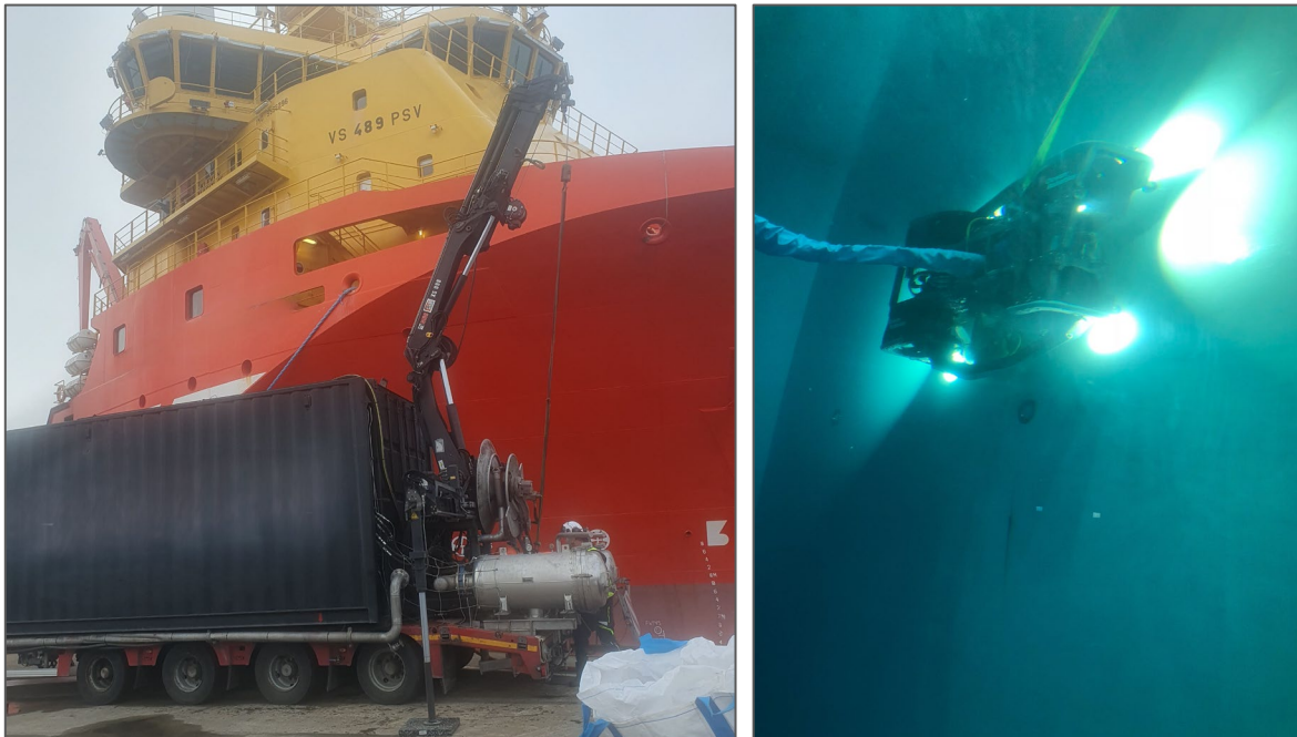
Figure 2. To the left: Petroleum service vessel and container unit for in-water hull cleaning. To the right: Cleaner ROV in action under water (Foto: Vivian Husa and Ecosubsea).
