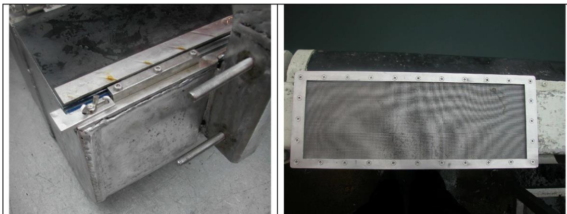
Left side: locking mechanism for the screen. Right side: screen with 0,5 mm mesh
