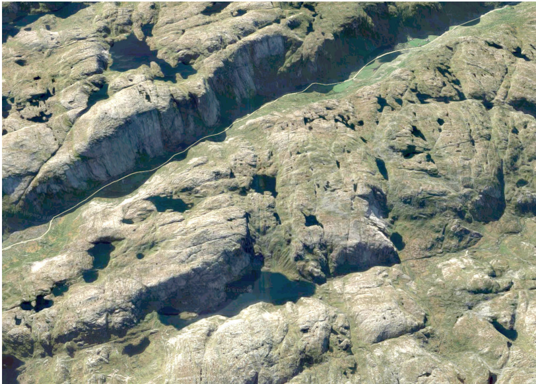
Fig. 5 Network of weakness zones in a mountainous area in southwest Norway. One can see the potential weakness zones as lines in the landscape due to glacial erosion. The depth of depressions is mainly a result of the rock quality, zone width and glacial motion direction. The road crossing the image is 10 km from edge to edge (Google Maps 2018).
