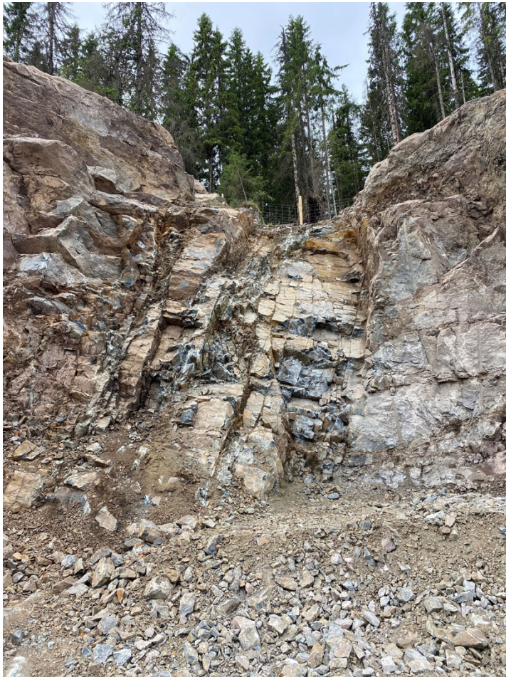
Fig. 6 Weakness zone in rhomb porphyry at the E16 Sandvika-Skaret project.
