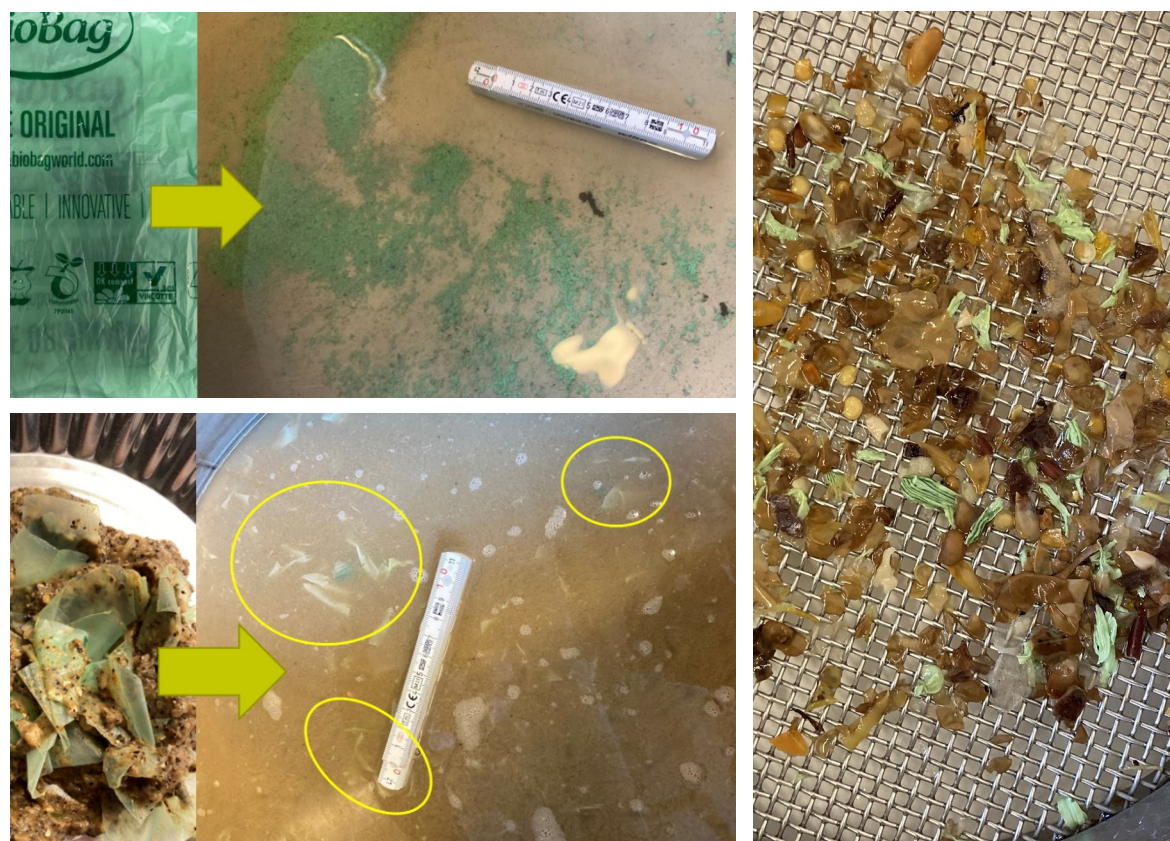
Figure 5. Left: Effect of THP on ICP alone (top) and in presence of food waste (bottom). Right: Recovered HCP together with food waste elements after THP (mesh size 2.5 mm).
