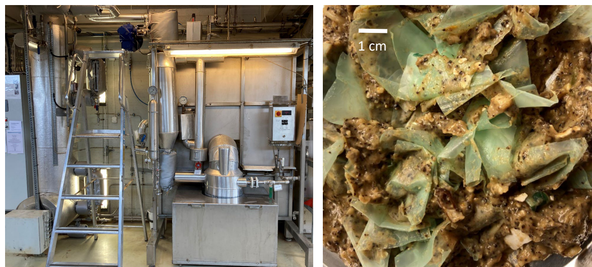
Figure 2. Thermal hydrolysis process (THP) unit used for pretreatment of biodegradable plastics, either on their own or mixed with food waste (as shown on the right picture).
