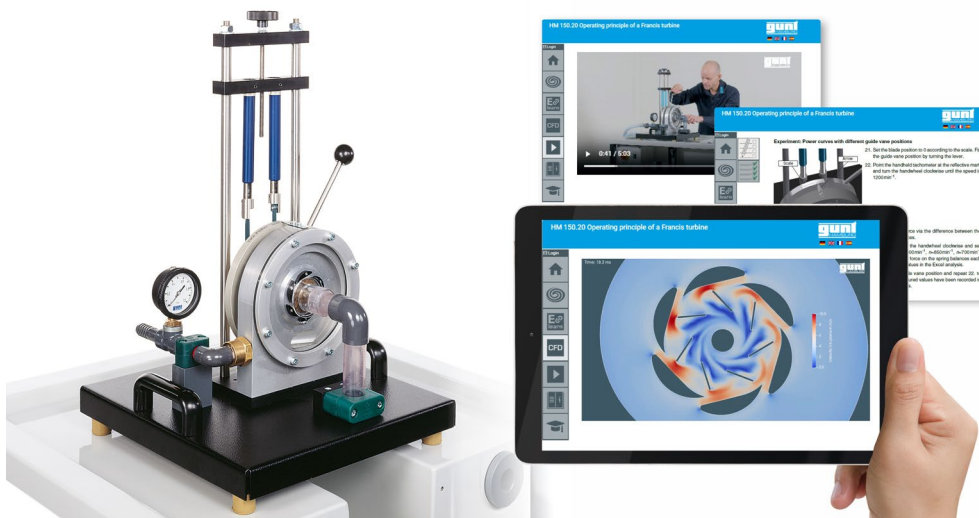
Figur 3: Modul for driftsprinsipp for en Francisturbin (H150.20)
