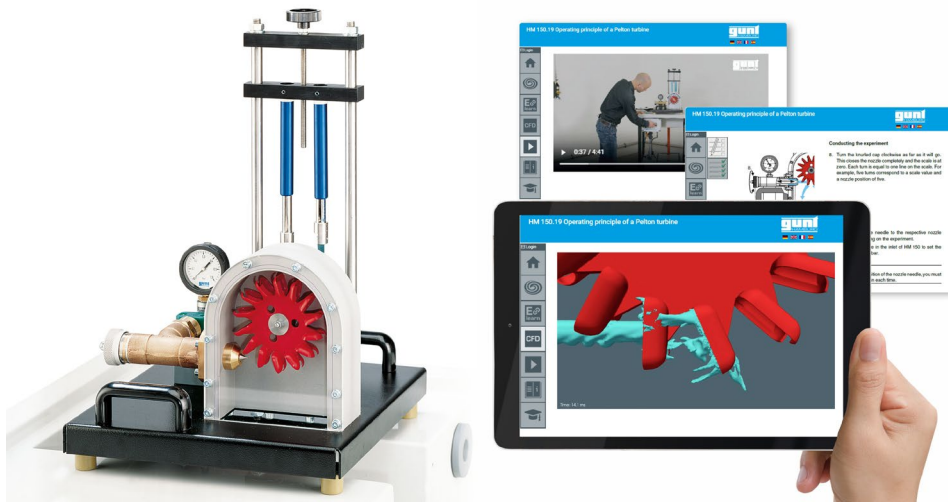
Figur 2: Modul for driftsprinsipp for en Pelton turbin (H150.19)
