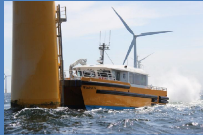
3 workboat access vessels for transferring technicians and transporting small components. the WindCat MKIII 10
