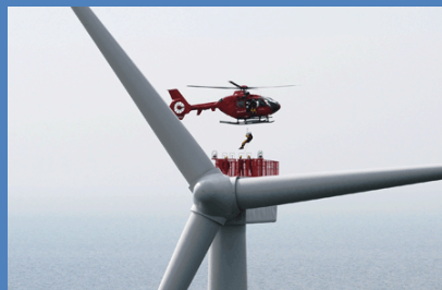
2 helicopters for transporting technicians for specific types of maintenance and emergency evacuation 13
