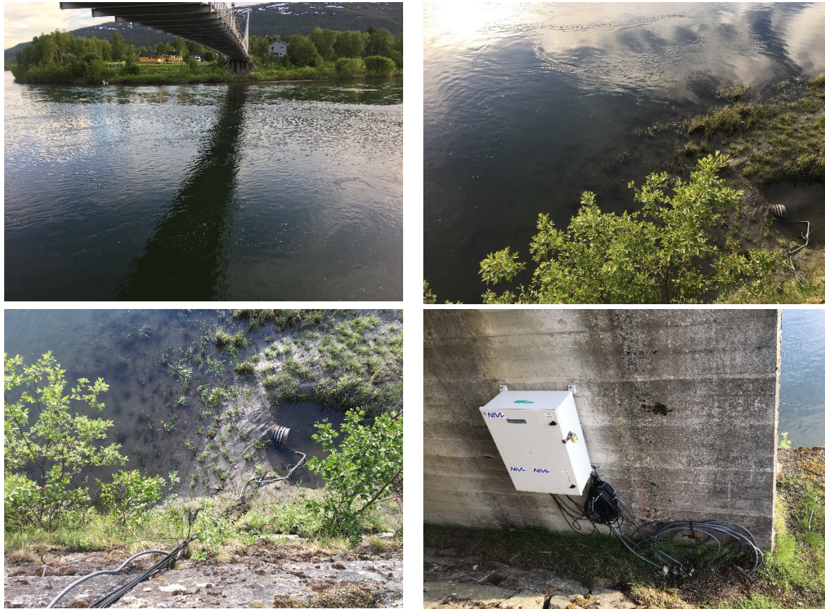
Figure A2. Photos from the Målselva sensor station showing the location of the sensor (near the old E6 bridge at Moen), location of the pipe through which sensors are deployed and the logger box.
