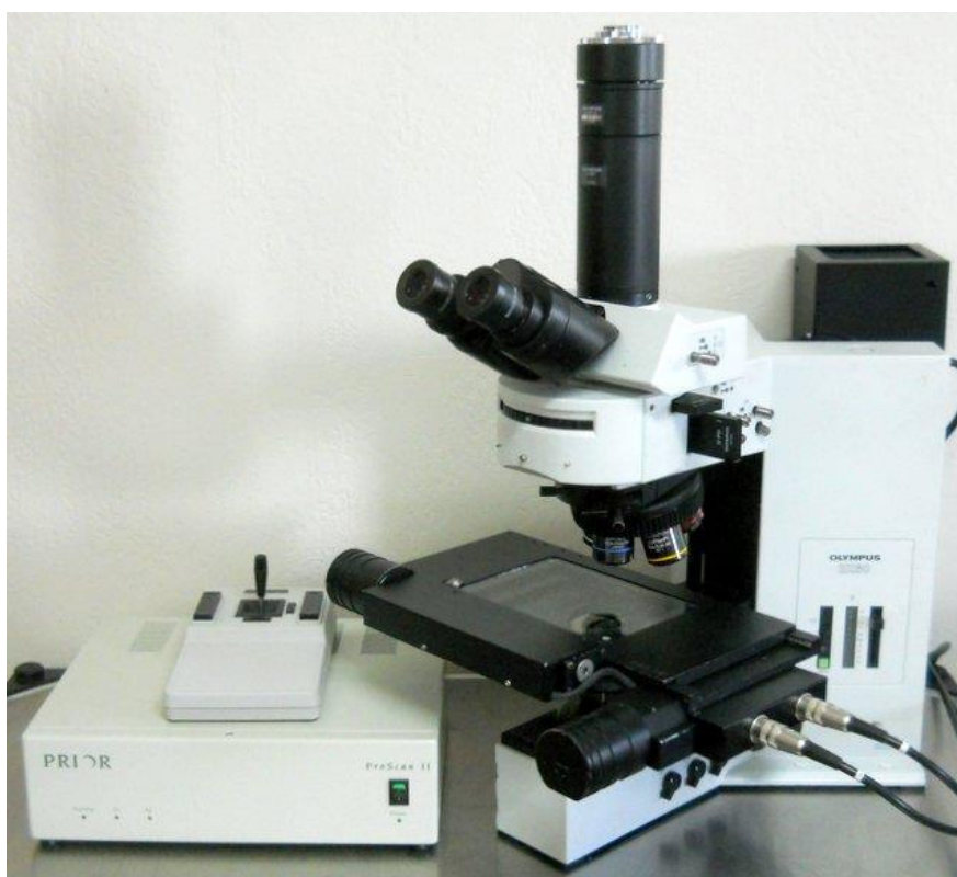
Figure 9-21: RGB Olympus BX60F5 Upright Metallurgical Microscope
