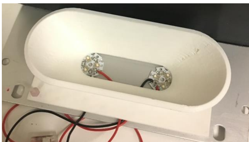
Figure 9-25: Light source of Industrial microscope version 1
