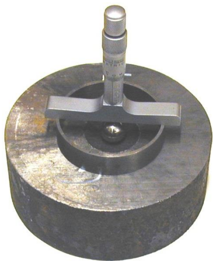
Figure 2.9 Picture of the tool used to measure the Dent depth.
