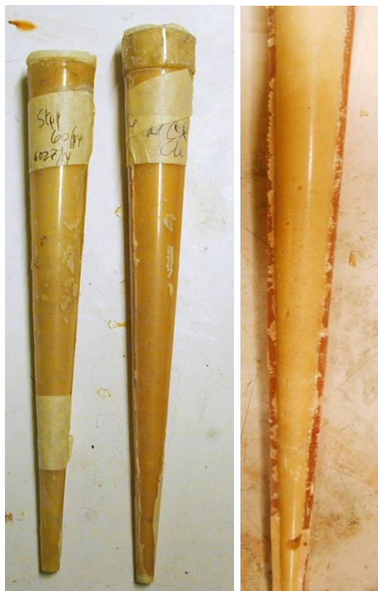
Figure 2.6 Picture of conical charge cast 60/14 to the left and cast 40/14 to the right together with a picture of the divided mould of cast 40/14.
