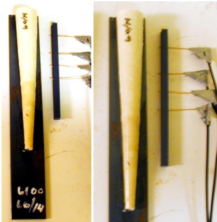
Figure 2.8| Pictures of conical charge 60/14 before assembled on the witness plate.
