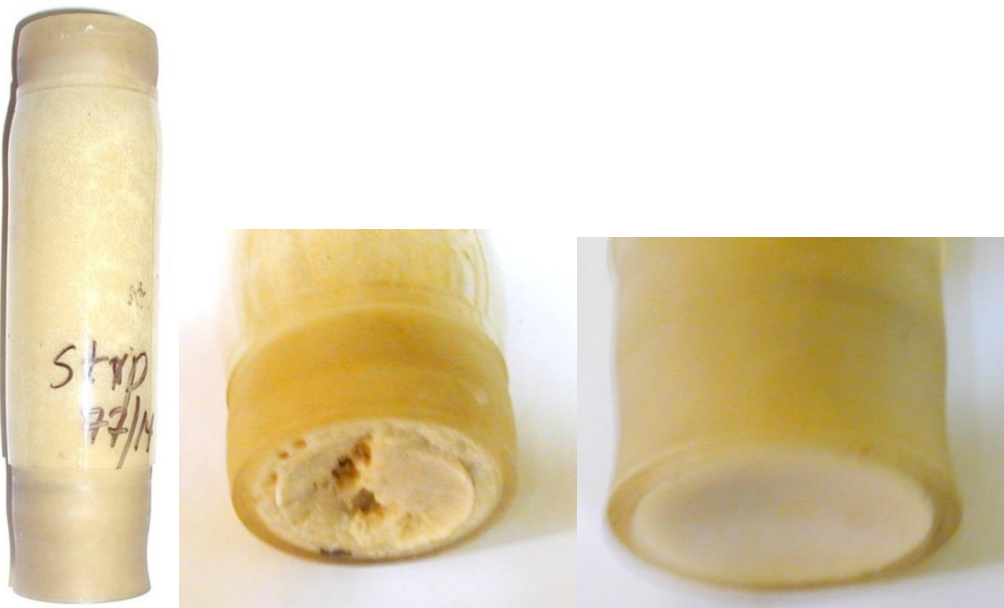
Figure 2.1 Casted charge to the left, the top in the middle and the bottom to the right.
