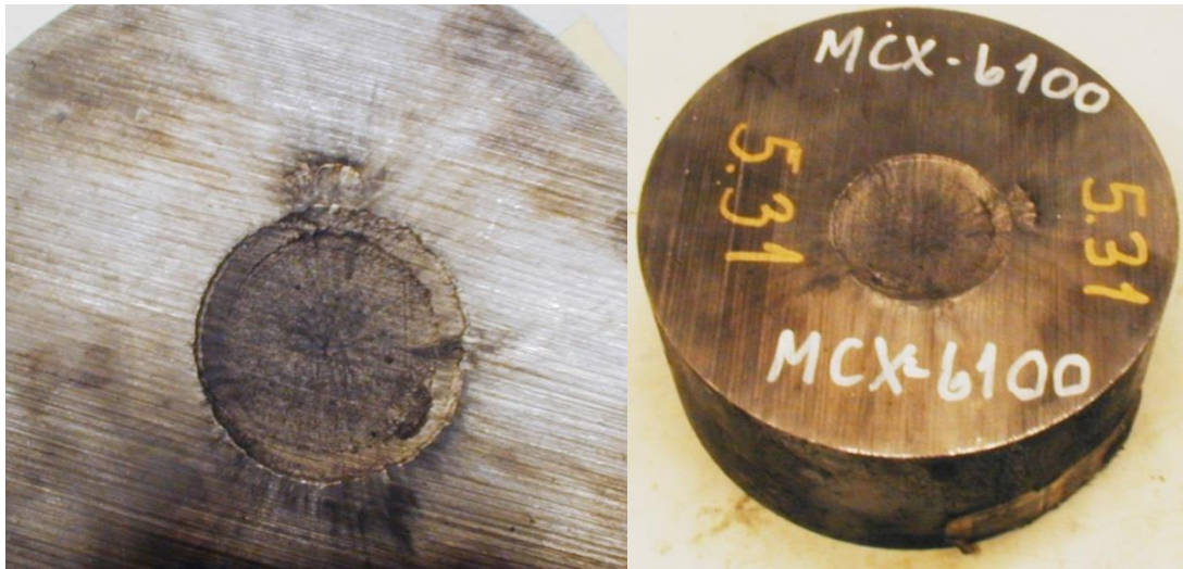
Figure 3.4 Pictures of the Dent plate after firing.
