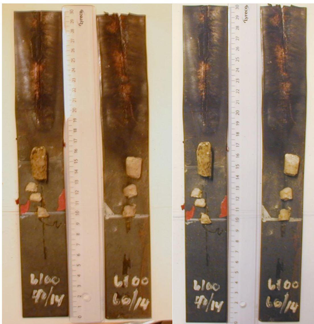
Figure 3.10 Pictures of the witness plates for MCX-6100 CH 6027/14 cast 40/14 and cast 60/14 included recovered unreacted explosive.
