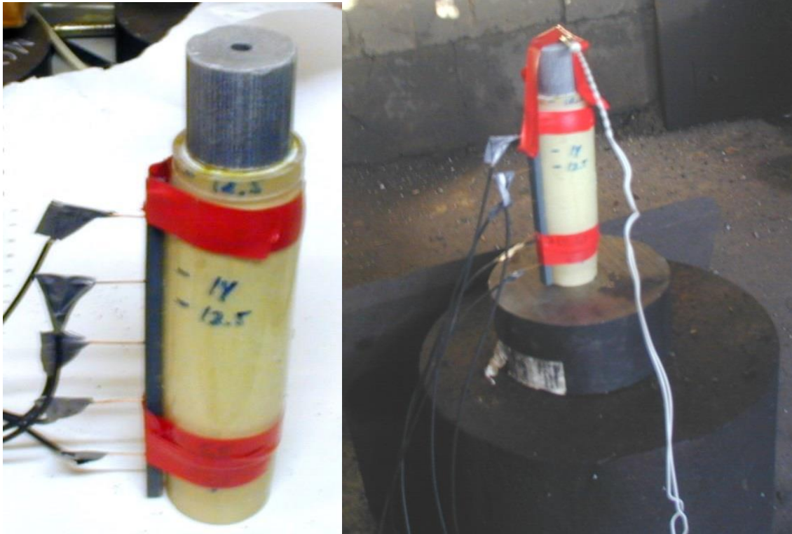
Figure 3.1 Pictures of the test charge before firing and test setup to the right.
