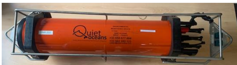
Figure 7: ORCA72D recorder in its mechanical protection frame
