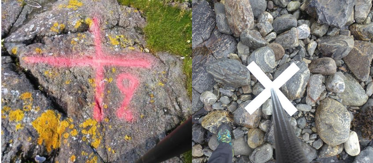
Figure 4. Ground control points (GCPs) were used to ensure correct geopositioning of the drone images. For the marking, either an environmentally friendly, soluble chalk paint (left) that disappears in less than 30 days or a portable and reusable wooden cross painted in white (right) was used. Photos (CC): Hege Gundersen (left) and Kasper Hancke (right).
