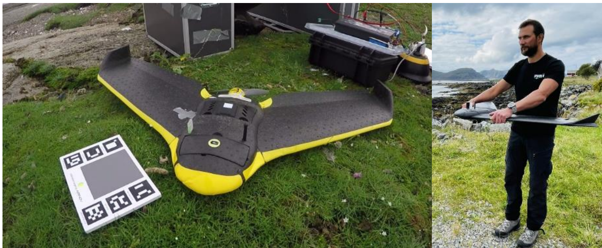
Figure 3. The fixed-wing drone used in the project, an eBee X mapping drone from AgEagle Aerial Systems. The drone was equipped with a multispectral imaging sensor (Micasense, Rededge-MX) that collected data in 5 specific color bands (see Table 1 for details). Photos (CC): Kasper Hancke.
