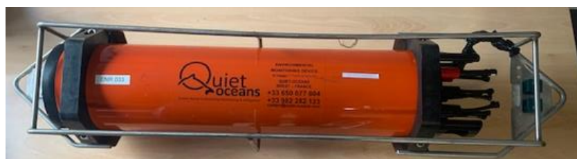
Figure 7: ORCA72D recorder in its mechanical protection frame
