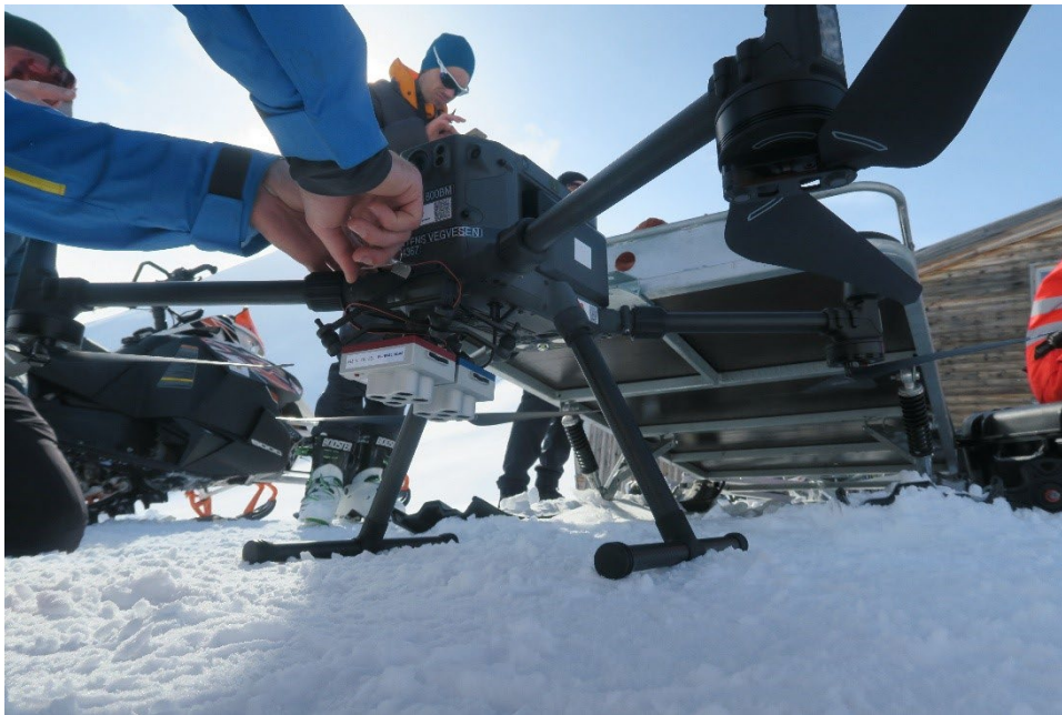
Figure 10: the MicaSense multispectral camera mounted on NPRA's DJI Matrice 300. An external GPS receiver was also mounted on the UAS for geotagging multispectral data. The camera was controlled directly from the ground via WiFi interface. (Photo: Tore Humstad)
