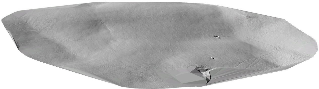
Figure 4: Hill-shaded terrain model (0,1x0,1 m cell size) based on the point cloud depicted in Figure 3.
