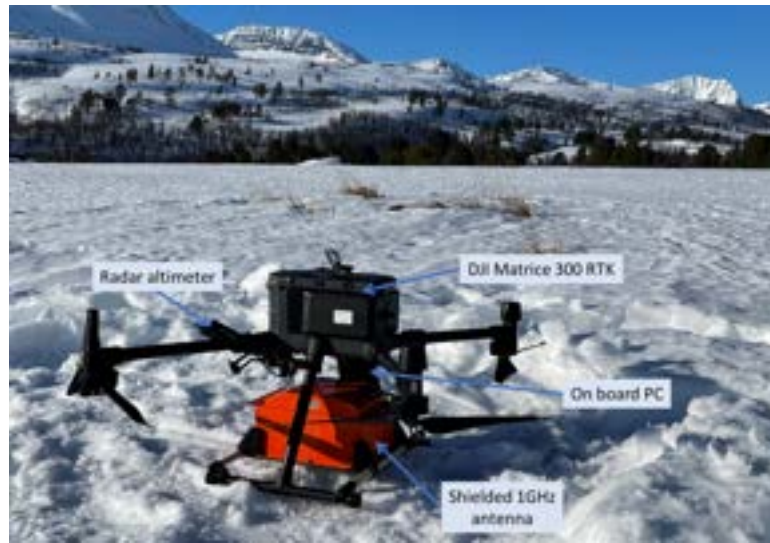
Figure 3: Picture of the high frequency system (1 GHz shielded antenna) mounted on a commercial UAV (DJI Matrice 300 RTK) and using a radar altimeter and onboard computer for terrain following and data logging (credit Sintef Industri)
