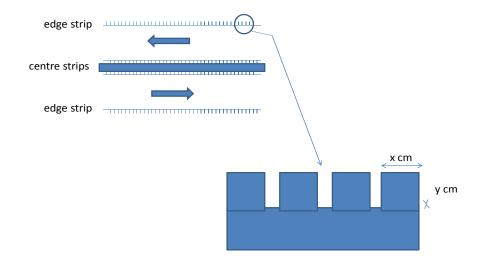
Figure 1. Typical rumble strips in Norway. The lengths x and y vary, but are typically either 6 or 10. "Longflex" strips are shown, but the lines can also be dippled or plain. Another common variant is an interrupted or 'dashed' rumble strip.
