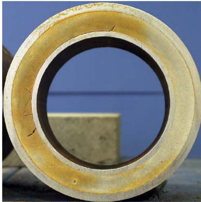
Figure 3.4: Damage (fractures) occurring in cyclic pressure testing of conventional cement in a test conducted by Halliburton (Heathman et al. (2006)).
