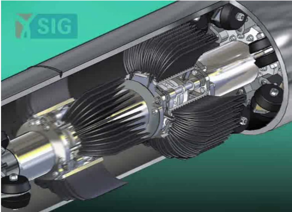
Figure 6.8. Illustration of guided wave inspection pig (Evans 2007).
