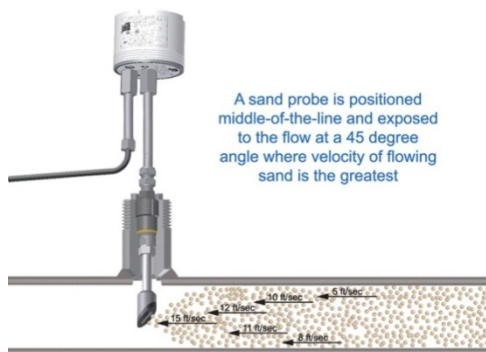
Figure 3.10 Rohrback Cosasco's Quicksand™ Erosion Detection System (courtesy Rohrback Cosasco).
