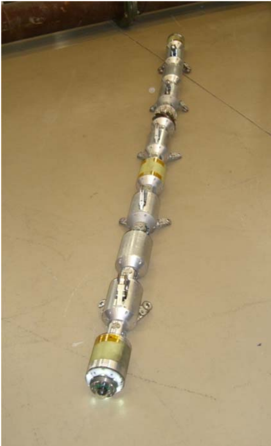
Figure 6.5. Pipeline crawler robot with RFEC inspection unit (Laursen 2009).
