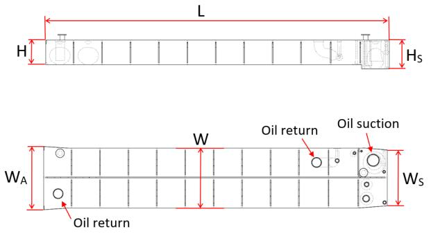
Figure 41: Side and top view of lube oil sump tank 5S, supplying DG4. Illustration: Fincantieri
