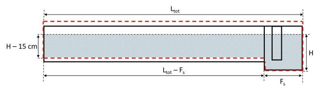
Figure 65: Oil volume calculated by use of the erroneous model for a given oil filling height "H". Illustration: NSIA
