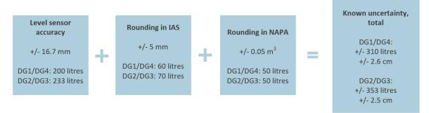
Figure 67: Known, total uncertainty for the remote monitoring system. Illustration: NSIA
