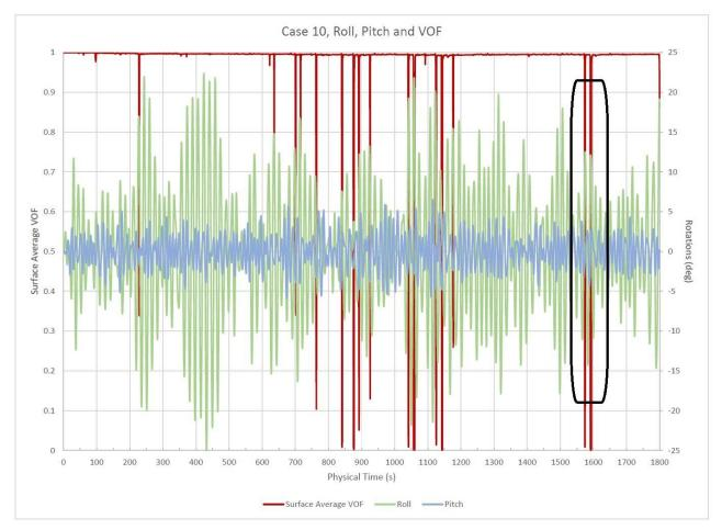
Figure 54: Graphical representation of results of CFD analysis from Lloyd's Register. Source: Lloyd's Register
