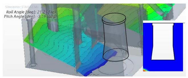
Figure 51: Illustration from the CFD simulation showing the suction pipe completely exposed to air. The multi-coloured surface represents the surface of the oil. The illustration in the box to the right shows a 2D side view of the suction pipe. Source: SINTEF Ocean/NSIA
