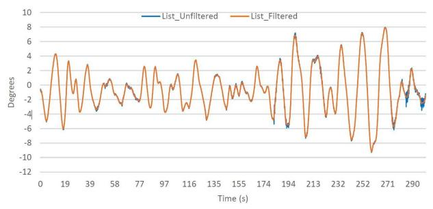
Figure 25: Angle of list (roll), filtered and unfiltered signal. Source: Eniram data / SINTEF Ocean's CFD report
