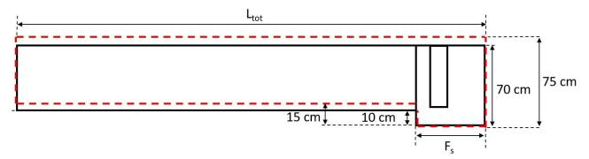
Figure 63: Actual tank (black contour) and the erroneous model (red dotted line). Illustration: NSIA
