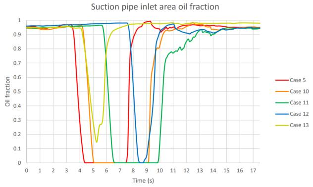
Figure 52: Oil fraction at suction pipe inlet area. Case 10 represents the worst case. Source: SINTEF Ocean's CFD calculation
