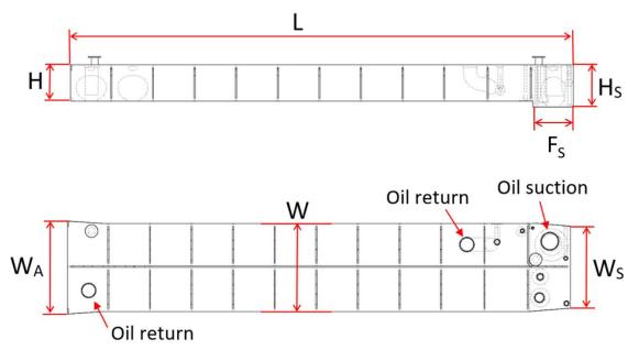
Figure 43: Side and top view of lube oil sump tank 5S, supplying DG4. Illustration: Fincantieri
