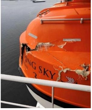
Figure 24: Damage to lifeboat on starboard side. Photo: NSIA
