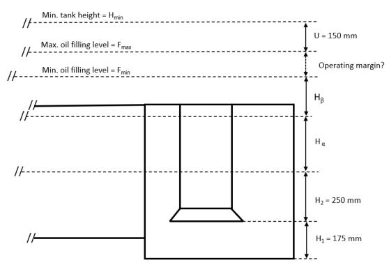
Figure 48: Minimum oil filling and tank height. Illustration: NSIA
