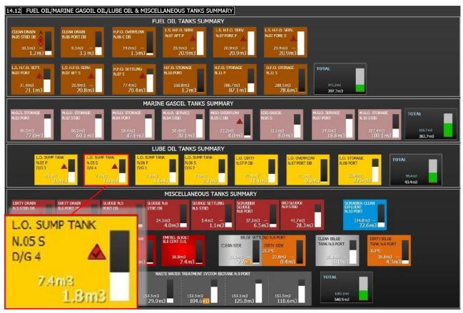
Figure 60: Extract from the tank mimics, showing the tank levels. Source: IAS/NSIA
