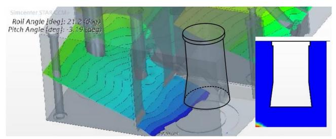
Figure 70: Illustration from the CFD simulation showing the suction pipe completely exposed to air. The multi-coloured surface represents the surface of the oil. The illustration in the box to the right shows a 2D side view of the suction pipe. Source: SINTEF Ocean/NSIA
