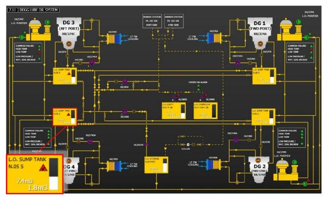
Figure 61: Extract from the lube oil system mimics, showing the tank levels. Source: IAS/NSIA
