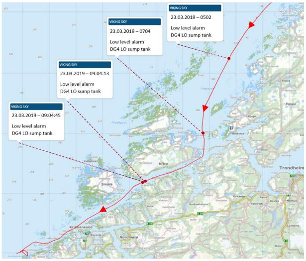
Figure 4: Lube oil sump alarms in the time period from 0502 until 0904. Illustration: The Norwegian Coastal Administration AIS / NSIA
