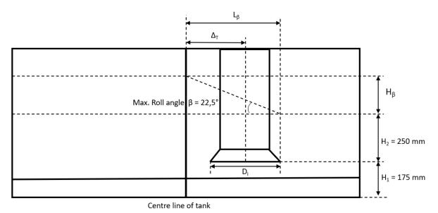
Figure 47: Dimensions relevant to calculate oil level reduction due to roll, H<sub>B</sub>. Illustration: NSIA
