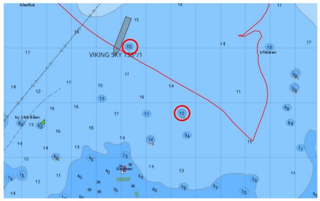
Figure 13: Viking Sky at 1427, drifting over a rock at a depth of 10 metres. Source: The Norwegian Coastal Administration AIS
