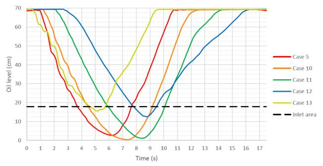
Figure 53: Oil level at suction pipe. Case 10 represents the worst case. Source: SINTEF Ocean's CFD calculation
