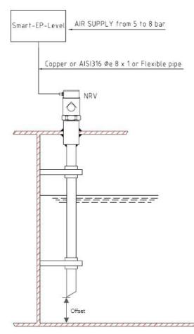
Figure 72: Illustration showing the physical offset. Extract: The system data sheet, S-SEPL-TM-V21. Rev. 20, Wärtsilä APSS srl.
