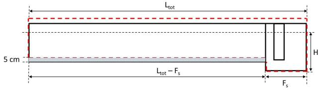
Figure 66: Difference in oil volume between a correct and the erroneous model. Illustration: NSIA
