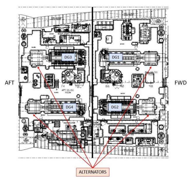
*Figure 28: Extract from the vessel's General Arrangement, showing the positioning of the DGs. Illustration: Fincantieri/NSIA*
