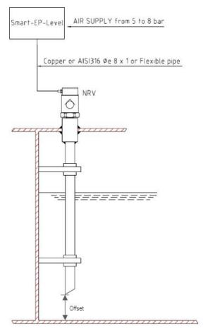
Figure 57: Installation of the level gauge system in the lube oil sump tank. Extract: The system data sheet, S-SEPL-TM-V21. Rev. 20, Wärtsilä APSS srl.
