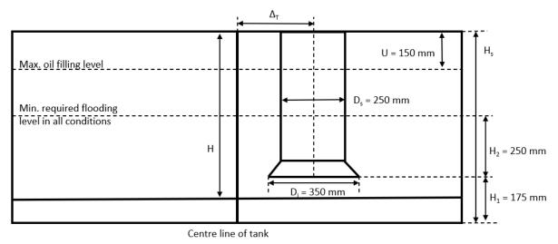
Figure 45: Transverse section view of suction end. Illustration: NSIA
