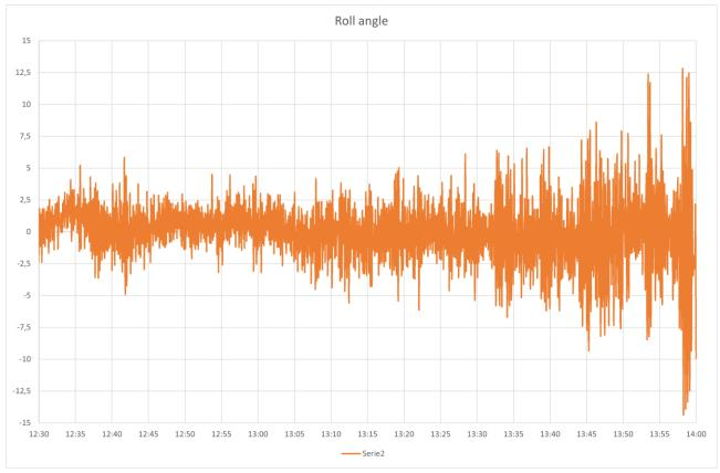
Figure 26: Roll angle registered by Eniram 1230 to 1400 LT. Source: Eniram/NSIA
