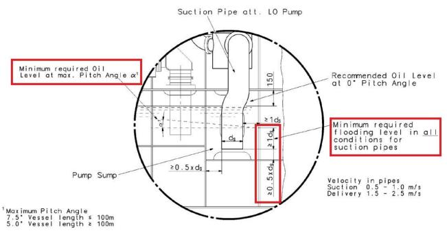
Figure 38: MAN project guide lubricating oil suction pipe detail. Extract: MAN
