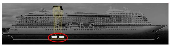
Figure 29: Viking Sky in profile, showing location of the DGs and the lube oil sump tanks. Illustration: Adobe Stock/Fincantieri/NSIA
