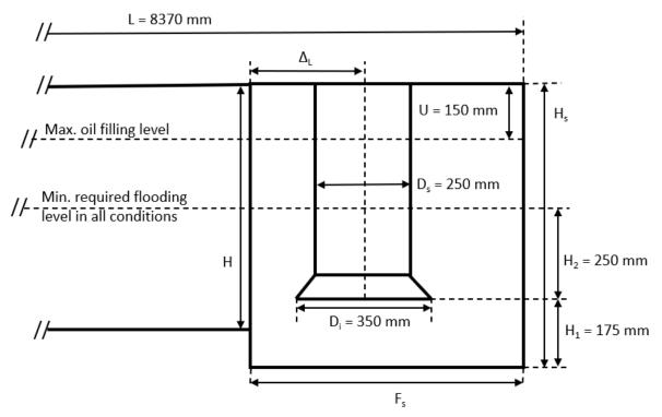
Figure 44: Longitudinal section view of suction end. Illustration: NSIA
