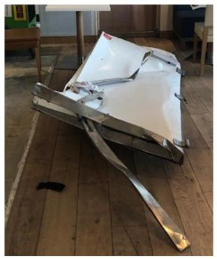
Figure 23: Broken door in the restaurant at deck 2. Photo: NSIA
