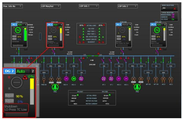
Figure 59: Extract from the power management mimics, showing the low lube oil alarm. Source: IAS/NSIA
