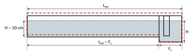
Figure 64: Actual oil volume for a given oil filling height "H". Illustration: NSIA
