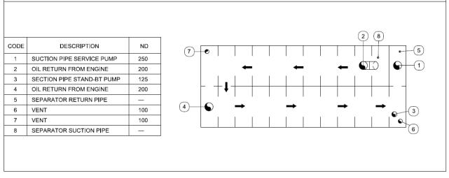
Figure 32: Extract from "Lube oil service system functional diagram", showing a sump tanks' baffle and pipework arrangement seen from above. Extract: Fincantieri
