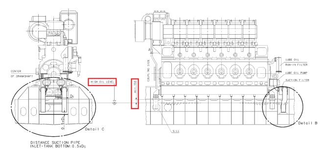
Figure 37: Extract from the MAN project guide showing the high oil level to be min 150 mm below the tank top. Extract: MAN
