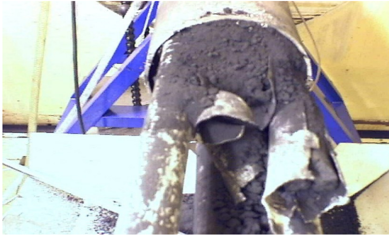
Figure 6-2. Corroded R1 fuel
