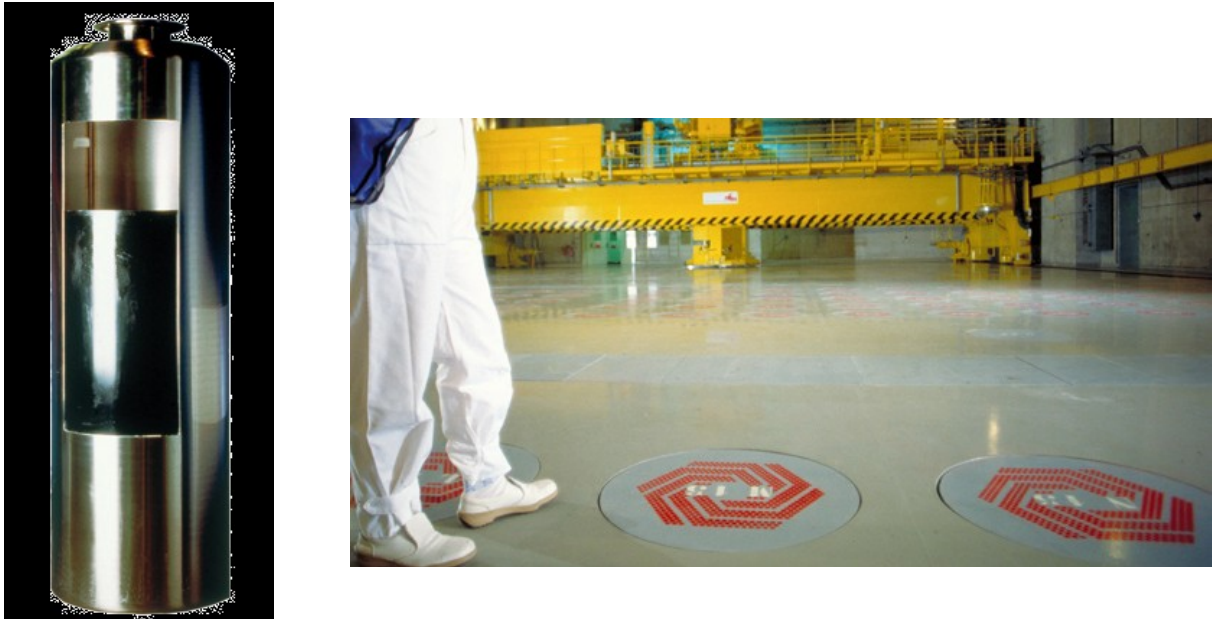
Figure 7-6. Vitrified waste canister and storage facility at Cap La Hague
