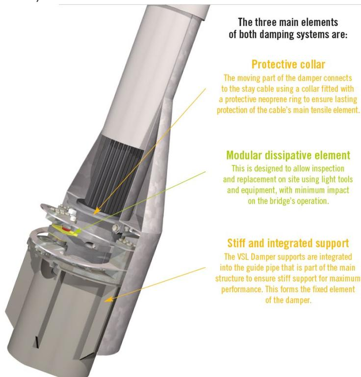
> Figure 7 Example of damper, VSL - friction damper
