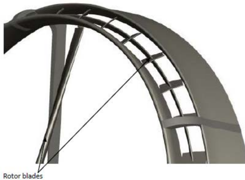
Figure 8: Part of the rotor and the outer rotor blade tips which will be rotating at high speed (Innowind)
