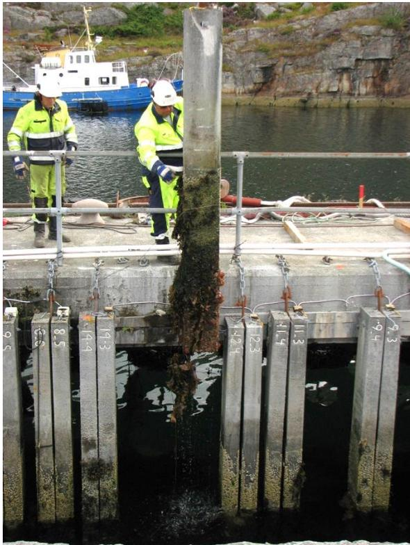
Figure 1: Lifting a pair of beams at the Solsvik field station for the extraction of cores (2013-08-12).
