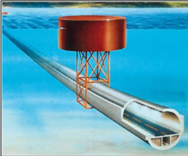
Figure 7 Submerged floating tunnel (<http://www.ntnu.no/gemini/1998-01E/36.html>)
