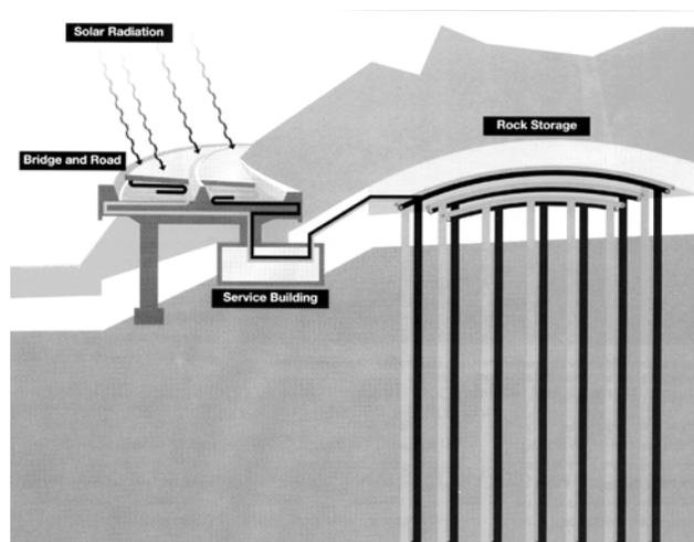
**Figure 11 A system of great interest if solar heated bridges are considered is the Swiss system reported by Rauber, 1995**
