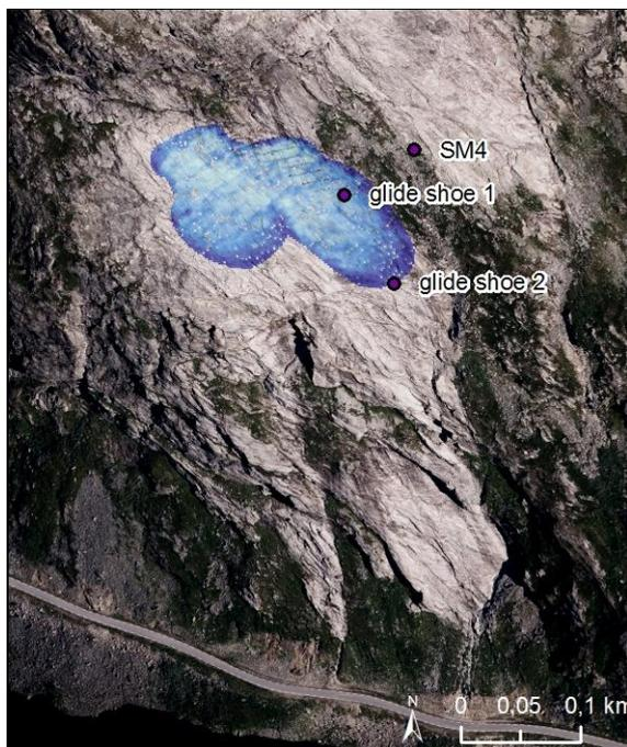
Figure 2: The field set-up around the Stabbrekka glide avalanche path shown on an aerial photo. The road is below. The blue shades correspond to areas with gliding snow in 2016. The upper limit correspond to the glide crack location, the lower limit correspond to the compression zone.
