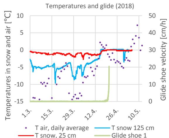
Figure 6: Temperatures from SM4 sensors and glide velocity from upper glide shoe in 2018
