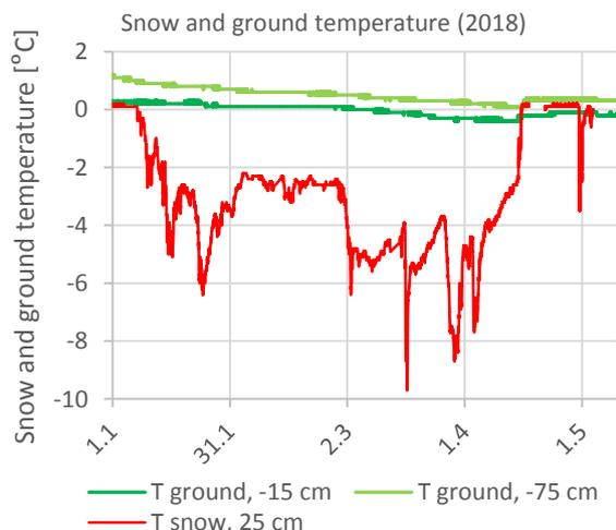
Figure 4: Temperatures at two depths in the ground and one height in the snow pack in 2018
