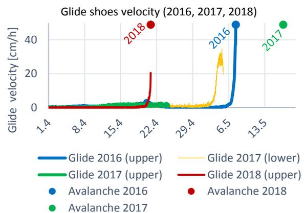
Figure 3: Monitored velocities at the upper (2016, 2017, 2018) and lower (2017) glide shoes combined with dates for the avalanches in the eastern slab.
