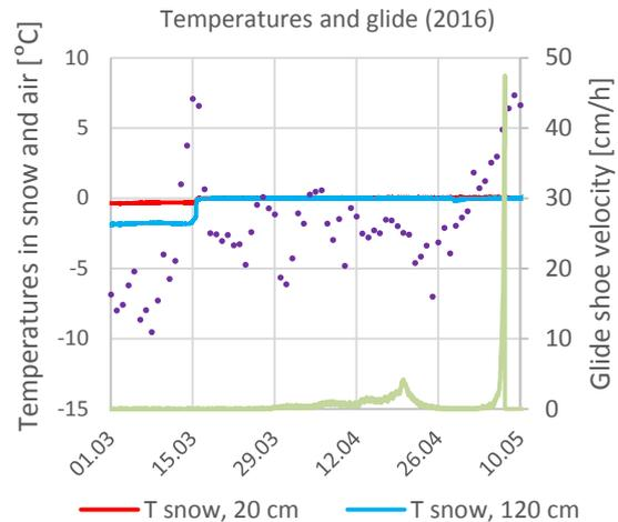
Figure 5: Temperatures from SM4 sensors and glide velocity from upper glide shoe in 2016
