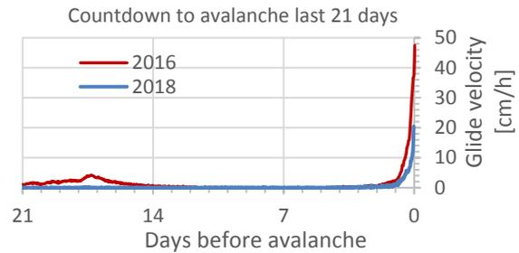
Figure 7: Glide velocity at glide shoe 1 the last 21 days, in retrospect, prior to the avalanches in 2016 and 2018
