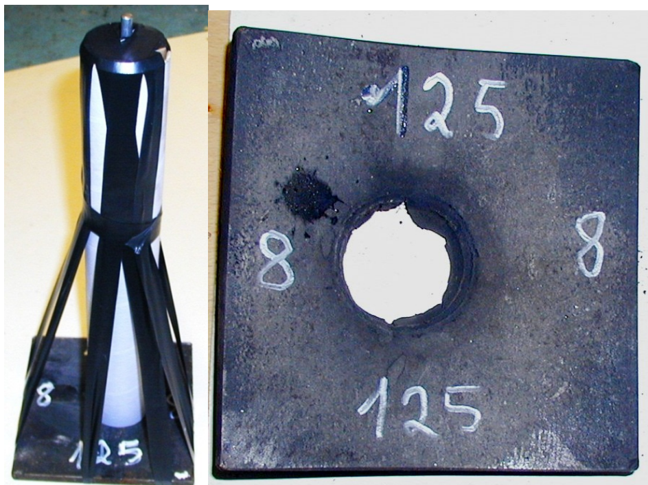
Figure 3.8 Pictures of tube No 8 before and after firing. Barrier thickness: 125 cards. Response: Detonation.
