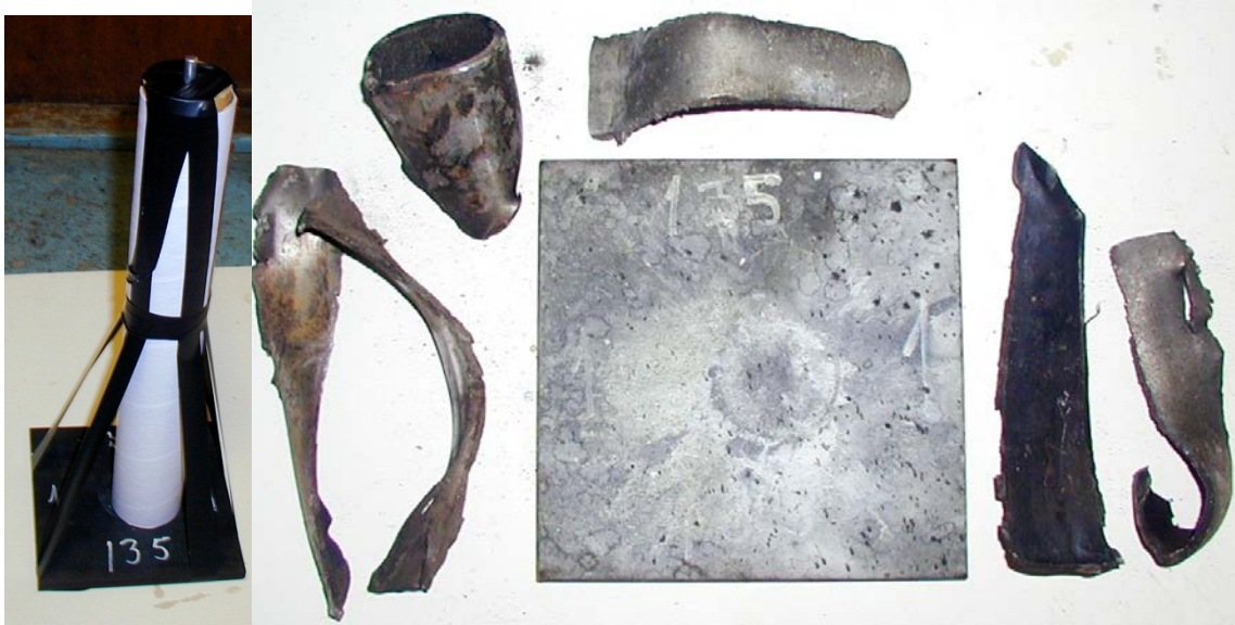
Figure 3.1 Pictures of tube No 1 before and after firing. Barrier thickness: 135 cards. Response: No reaction.
