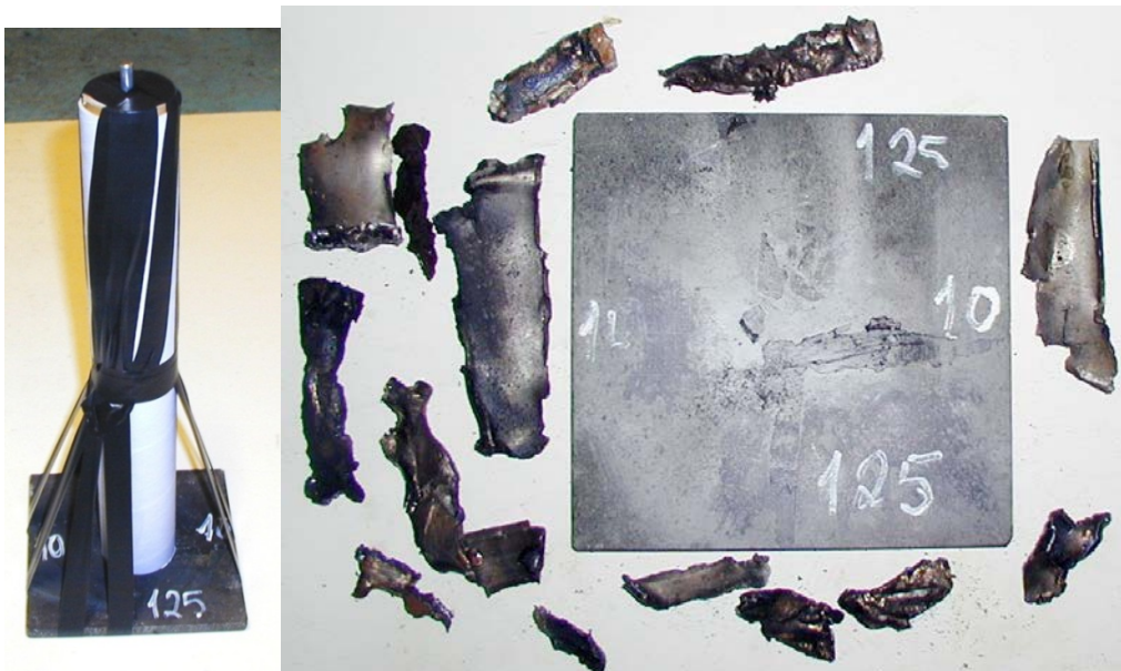
Figure 3.10 Pictures of tube No 10 before and after firing. Barrier thickness: 125 cards. Response: No reaction.
