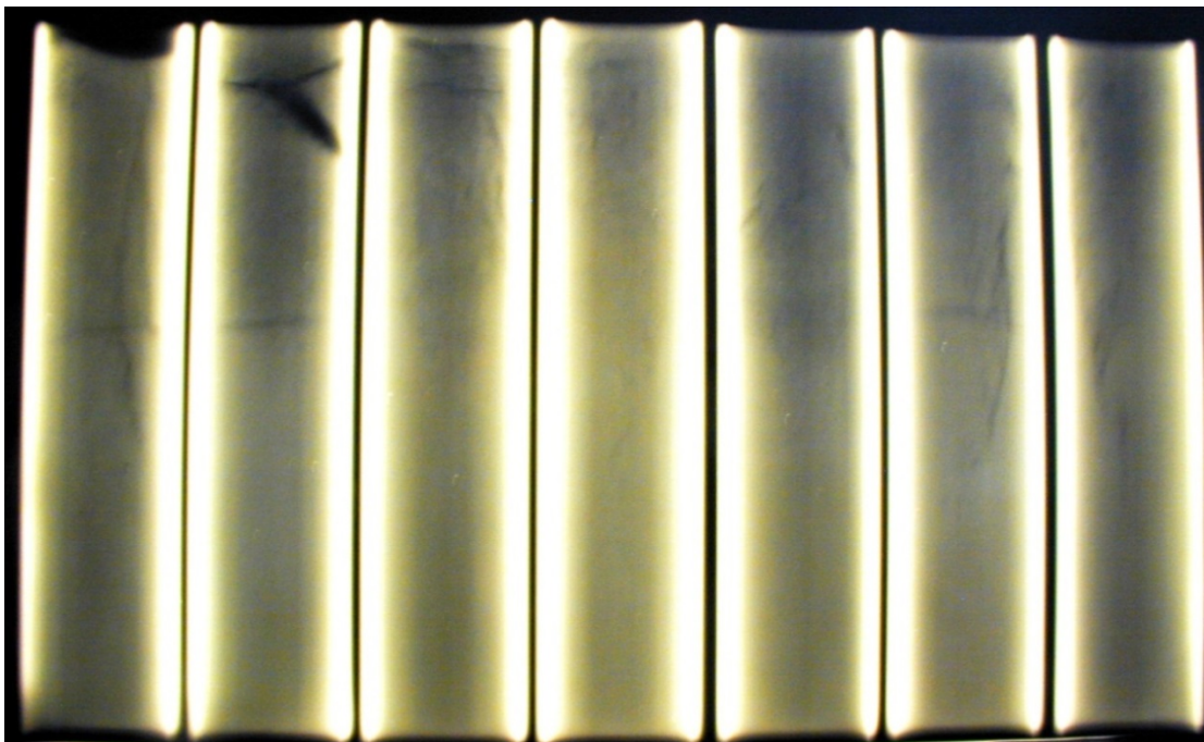
Figure 2.6 X-ray picture of tubes No1 to No 7 after being turned 90^\circ .
