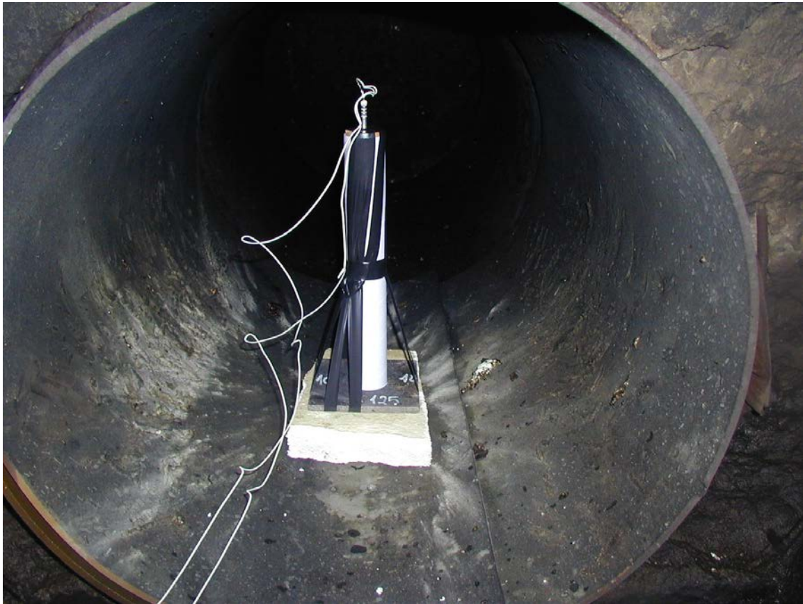
Figure 2.8 The picture shows the test setup used for firing of the Intermediate Scale Gap Test.
