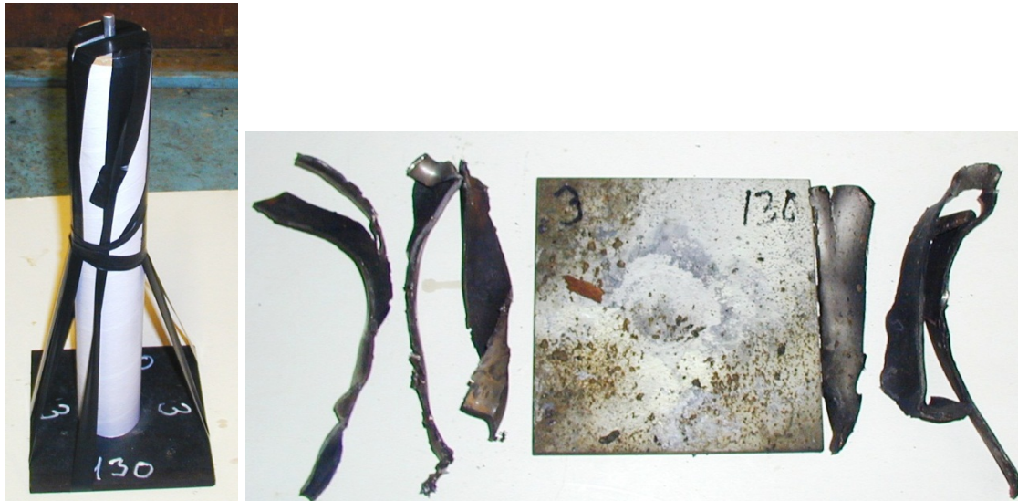
Figure 3.3 Pictures of the tube No 3 before and after firing. Barrier thickness: 130 cards. Response: No reaction.
