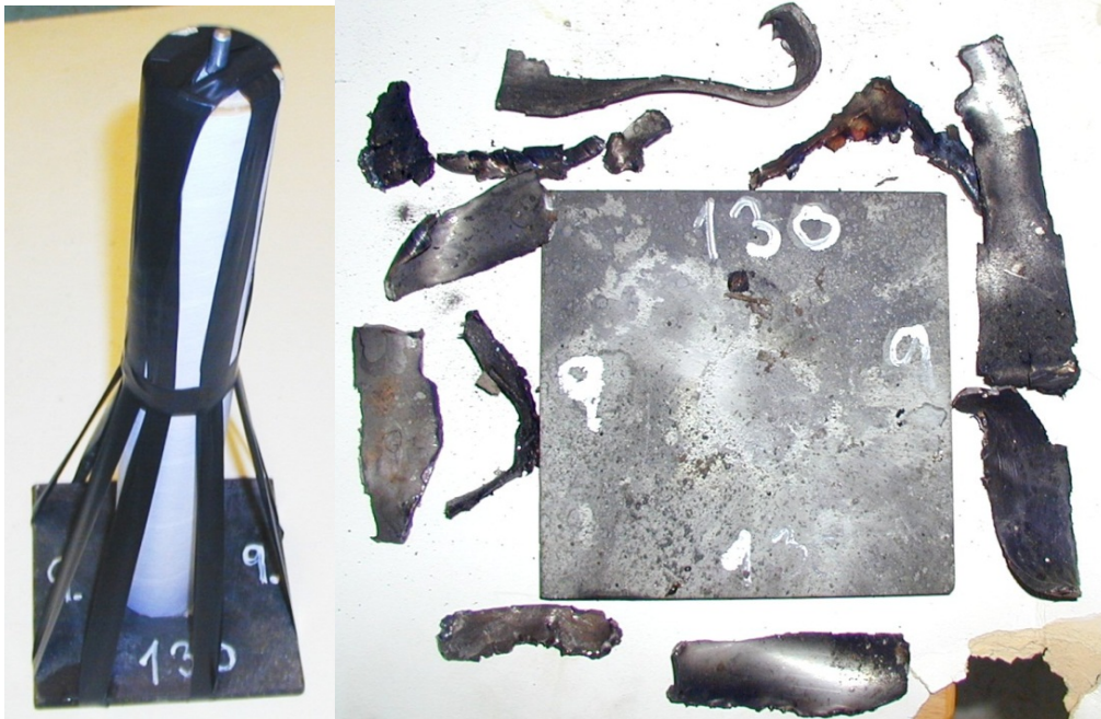
Figure 3.9 Pictures of tube No 9 before and after firing. Barrier thickness: 130 cards. Response: No reaction.
