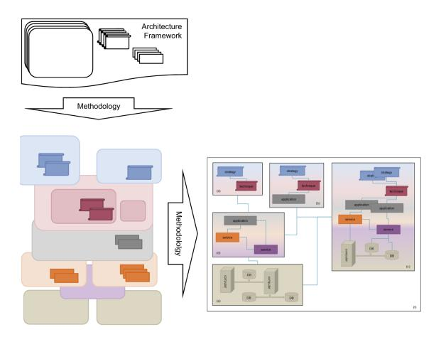
*Figure 2.1* Methodologies are used to transform between an architecture framework, an architecture and an actual system, shown here as a complex system-of-systems.
