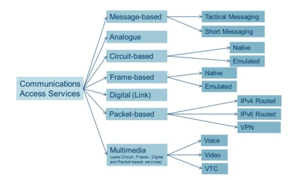
Figure 3.4 Decomposition of Communications Access Services.
