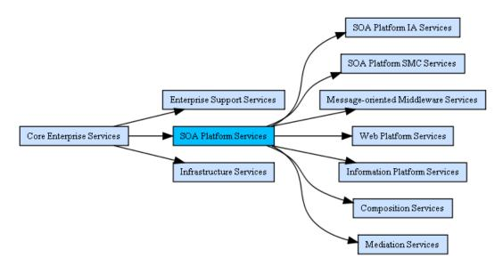
Figure 3.2 Decomposition of SOA Platform Services, from the C3 Taxonomy Enterprise Mapping.
