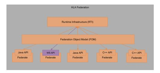
Figure 4.2 High-Level Architecture (HLA).
