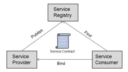
Figure 2.3 The SOA Triangle, which shows the relationship between the main SOA entities.
