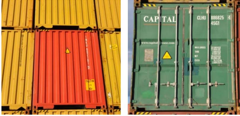
Figure 3.16 Differences between the front and back short sides of the container
