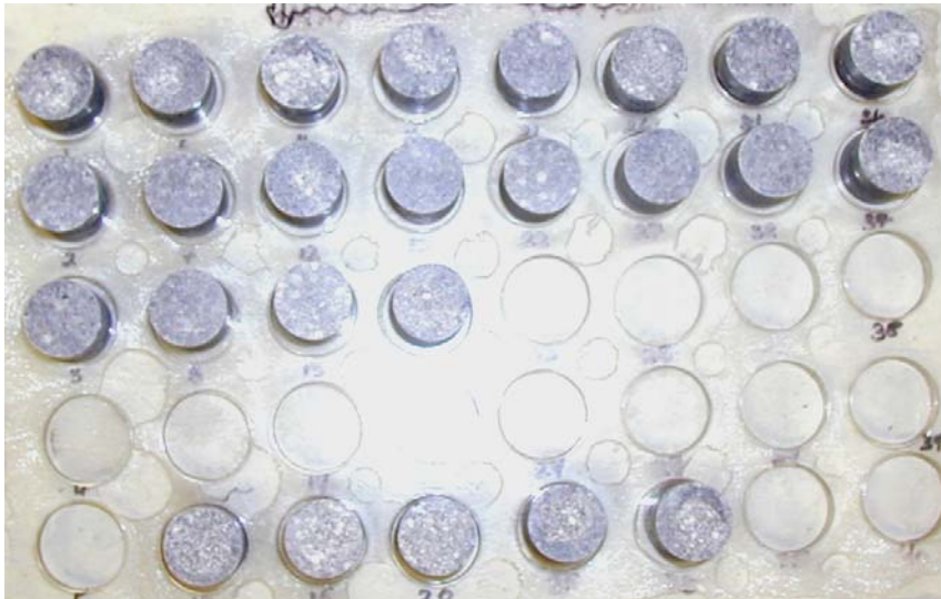
Figure 2.2 Picture of PBXW-11 pellets before start of ageing
