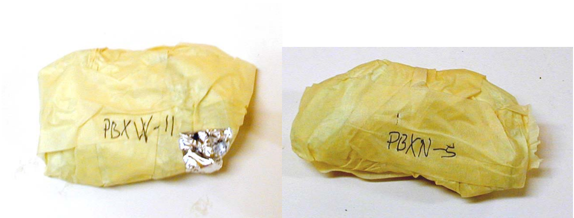
Figure 2.4 Picture of PBXW-11 pellets after they were packed in aluminum foil.
