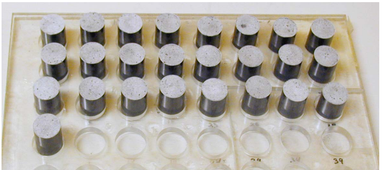
Figure 2.1 Picture of PBXN-5 pellets before start of ageing.
