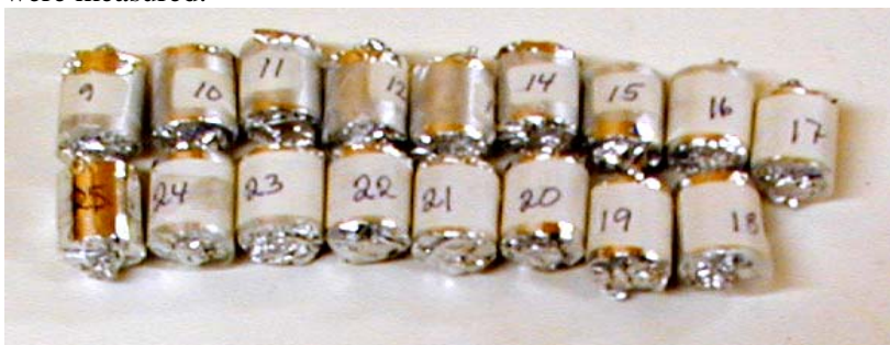
Figure 2.3 Picture of PBXN-5 pellets after they were packed in aluminum foil.
