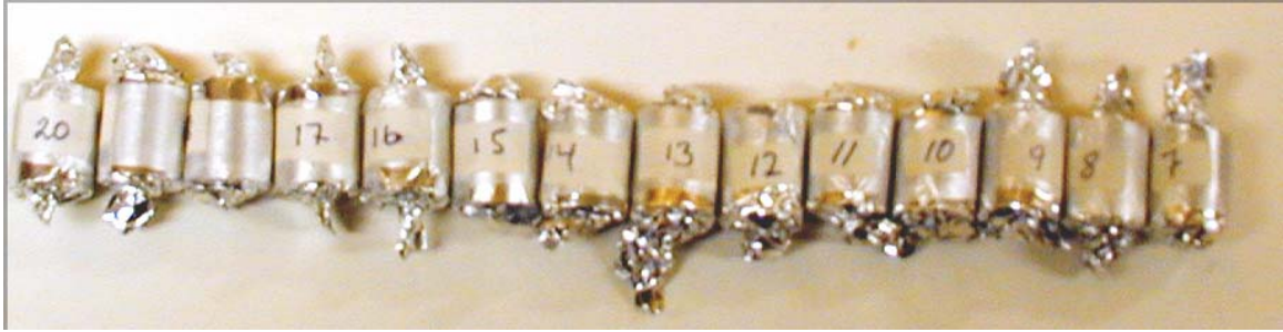
Figure 2.4 Picture of PBXW-11 pellets after they were packed in aluminum foil.
