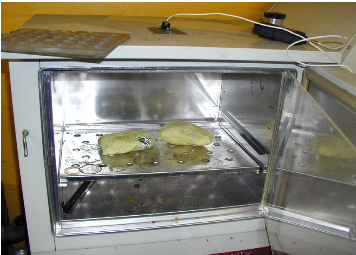
Figure 2.5 The picture shows the oven used to age the pellets. The upper part of the Figure gives pictures of how the pellets were packed during the ageing.
