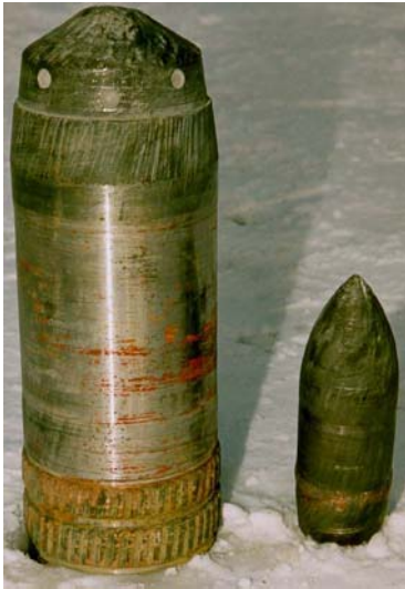
Figure 4.5 152 mm projectile (left) and 75 mm projectile used in the HPC and ANNC experiments.
