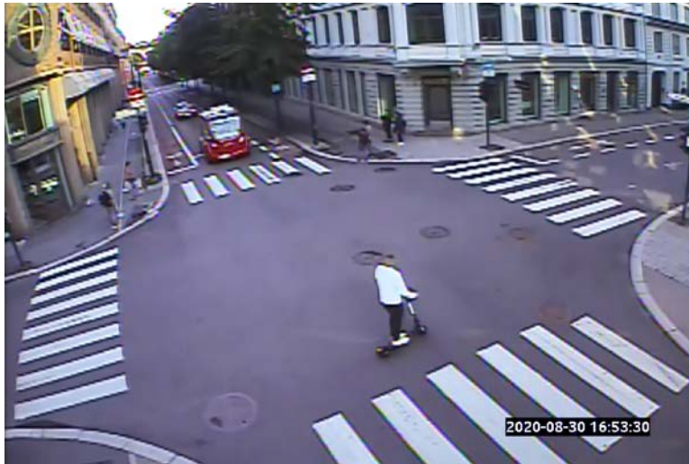
Figure 16 - El-scooterist entering Zone 3 on a red signal triggered the shuttle to stop (the reaction occurred in the position captured on the photo).
