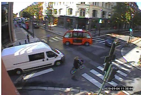
Figure 21 - The shuttle stayed inside the intersection after an unnecessary stop in Zone 3
