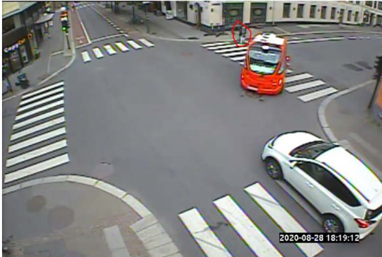
Figure 8 – Pedestrians (in red circle) starting to cross slightly outside the zebra crossing, the shuttle drives first
