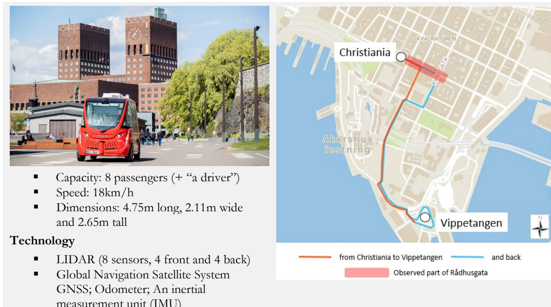
Figure 1 - The parameter of the shuttle (left, source: www.ruter.no ) and the studied route (right)
