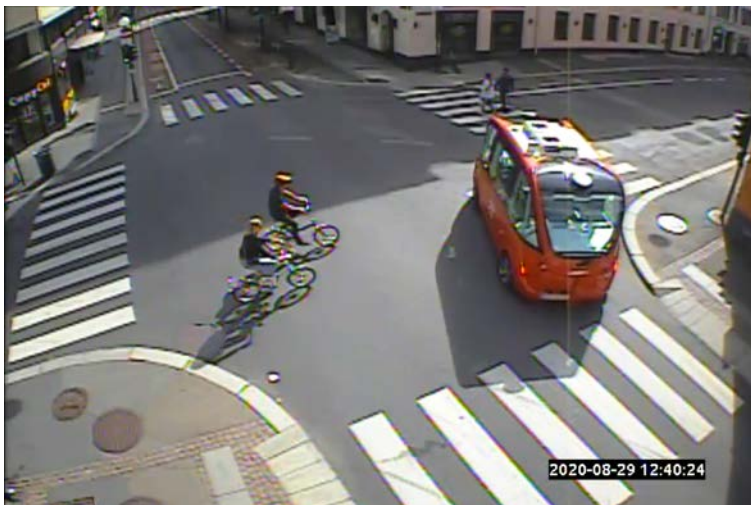
Figure 9 – Here, the shuttle had to deal with pedestrians crossing the zebra on green light, at the same time as cyclists approached from the left on red signal.
