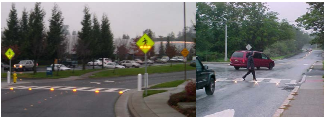
Figur 2.3.5: Fotgjengeraktivert asfalthys og blinklys på fotgjengerovergangskilt (venstre: http://honolulu.legalexaminer.com/automobile-accidents/the-pedestrian-crosswalk-safety-chronicles-innovative-solution-for-crosswalk-safety/ ; høyre: http://www.lrc.rpi.edu/programs/partners/partnersOnly/pdfs/CrosswalkSafety.pdf ).
