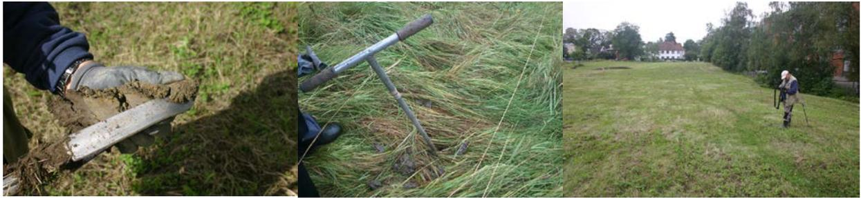
**Figure 6: (left to right) topsoil layer in an auger, an auger hole, and data digitalization (Photos: Cristina Gil Ruiz / NIBIO).**
