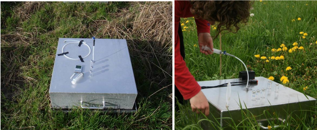
Photo 3.1 Non-steady state closed gas chamber installed in the arable land of south eastern Norway (left photo) and grassland in western Norway (right photo) fields (photo taken by Mehreteab and Sissel).
