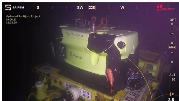
(b) Saipem's Hydrone-R med Subsea Docking Station (SDS) fra BlueLogic 13, 14 .
