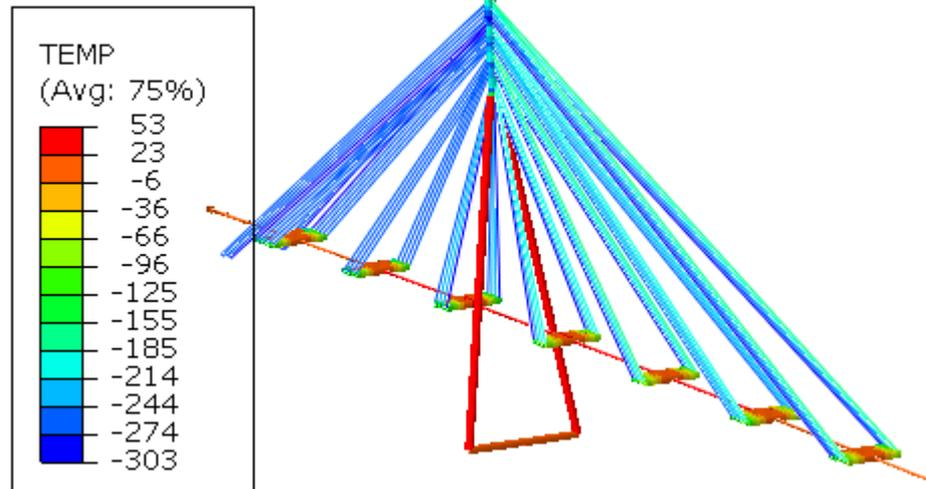
> Figure 4-5 Post tensioning of cables and elongation of girder and tower with temperatures [K].
