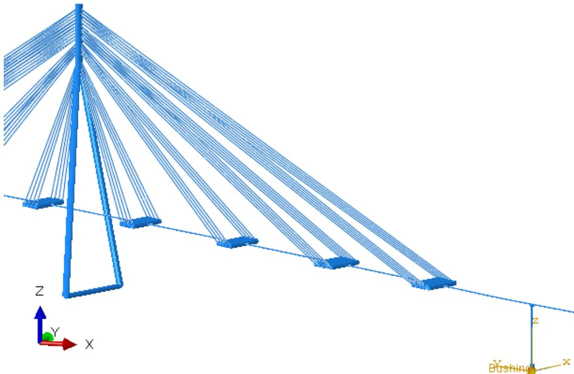
> Figure 4-2 Global FE-model showing area around the navigation channel. Beam profiles for tower, girder and pontoon columns are rendered.
