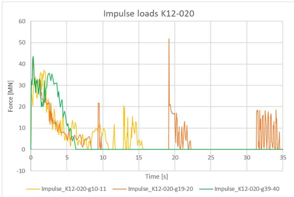
> Figure 5-2 Relevant impulse loads on bridge K12.
