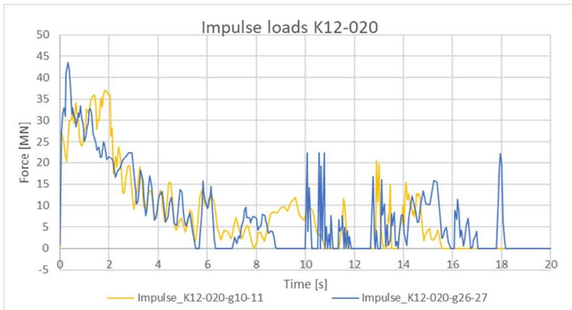
➤ Figure 5-6 Compared impulse loads on impacts g10-11 and g26-27
