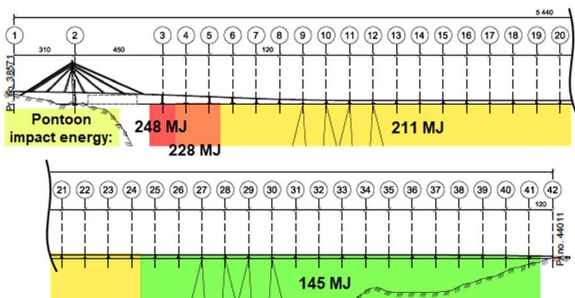
> Figure 2-1 Numbering of axis referring to pontoons and distribution of pontoon impact energy, see also Figure 3-2 for details. From drawing SBJ-33-C5-OON-22-DR-001.
