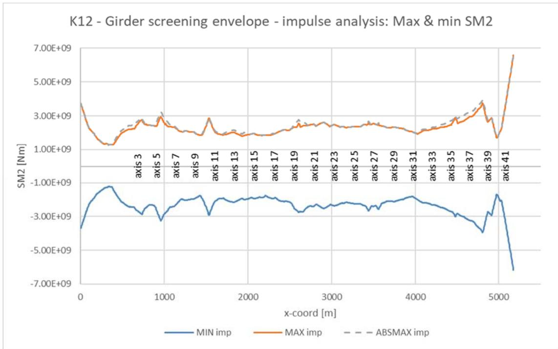
> Figure 5-3 Max and min envelopes for strong axis bending moments (SM2), [Nm]
